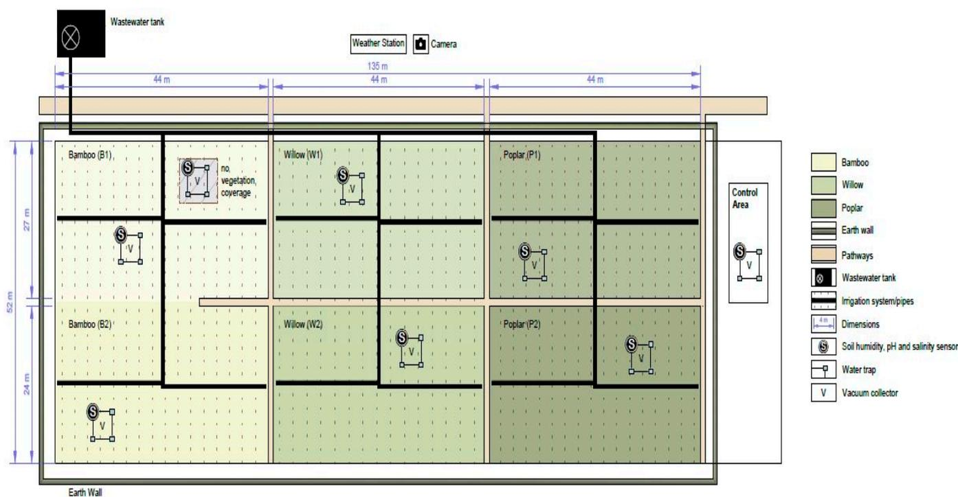
**Figure 5.** Design of the pilot wfsRC system at the AMU facilities in Aligarh.
