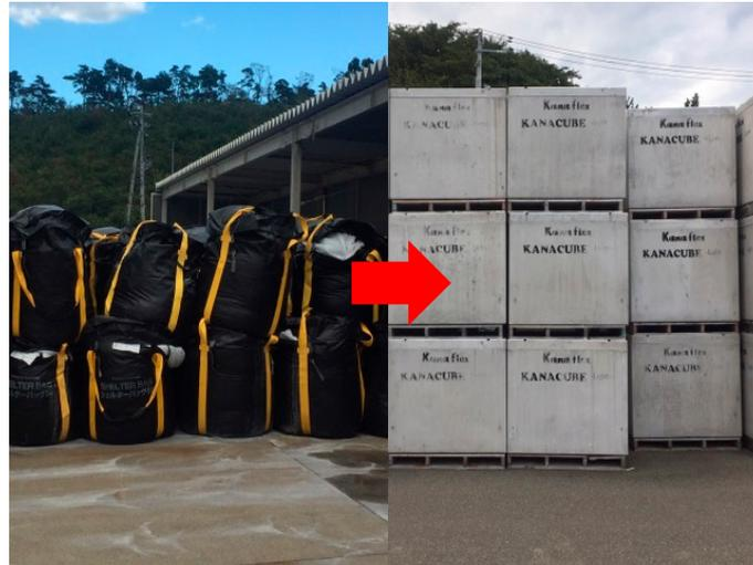
**Figure 5.** Example of temporary (left) and long-term (right) ash storage conditions in an MSW incineration facility.
