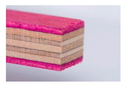
Figure 7. Face Wise Strip Orientation.
