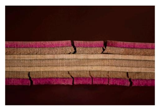
Figure 17. Cross Section View Showing Splitting in Sample 2.
