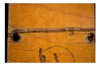
Figure 19. Top View Showing Splitting in Sample 1.
