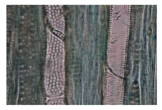
**Figure 25.** Tangential view of face veneer showing alternate intervessel pitting, spiral thickenings, and cross section of sample perforation plates (400×) that are characteristic of sugar maple (Acer saccharum).
