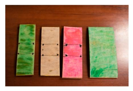
Figure 12. Bottom view of samples after soak/dry moisture durability test (ANSI/HVPA EF 2009 [4]).
