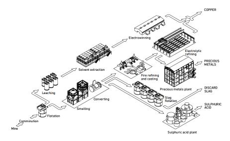
Figure 1. The process routes of primary copper production [10].
