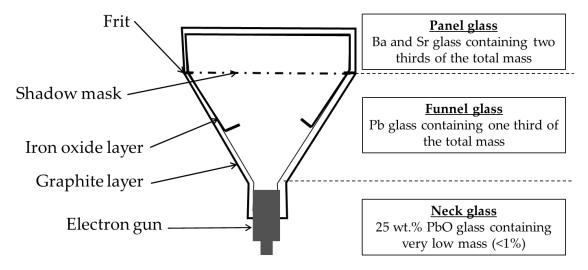
**Figure 1.** Schematic diagram showing CRT components: the panel glass, funnel glass, and neck glass, with brief information on each section.
