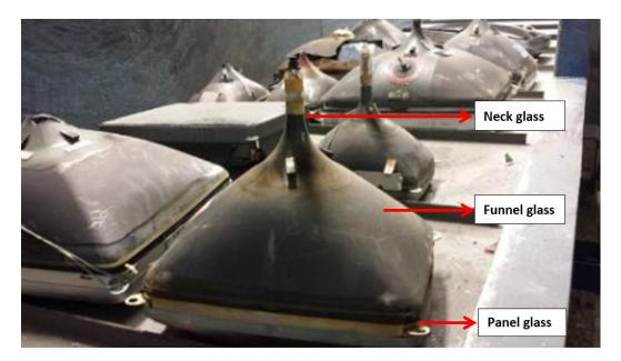
Figure 4. Stripped CRT monitors.
