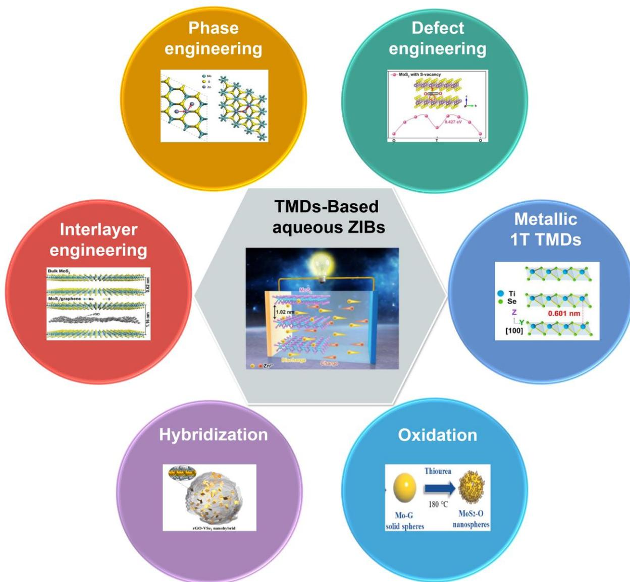
**Scheme 1.** Schematic of the effective strategies for optimizing the  $\text{Zn}^{2+}$  storage ability and cycling performance of TMD-based ZIB cathodes. Reprinted with permission from Refs. [13–18]. Copyright 2021, Wiley-VCH GmbH, Weinheim. Copyright 2020, Elsevier. Copyright 2021, Wiley-VCH GmbH, Weinheim. Copyright 2020, Elsevier. Copyright 2021, Elsevier. Copyright 2021, Elsevier.
