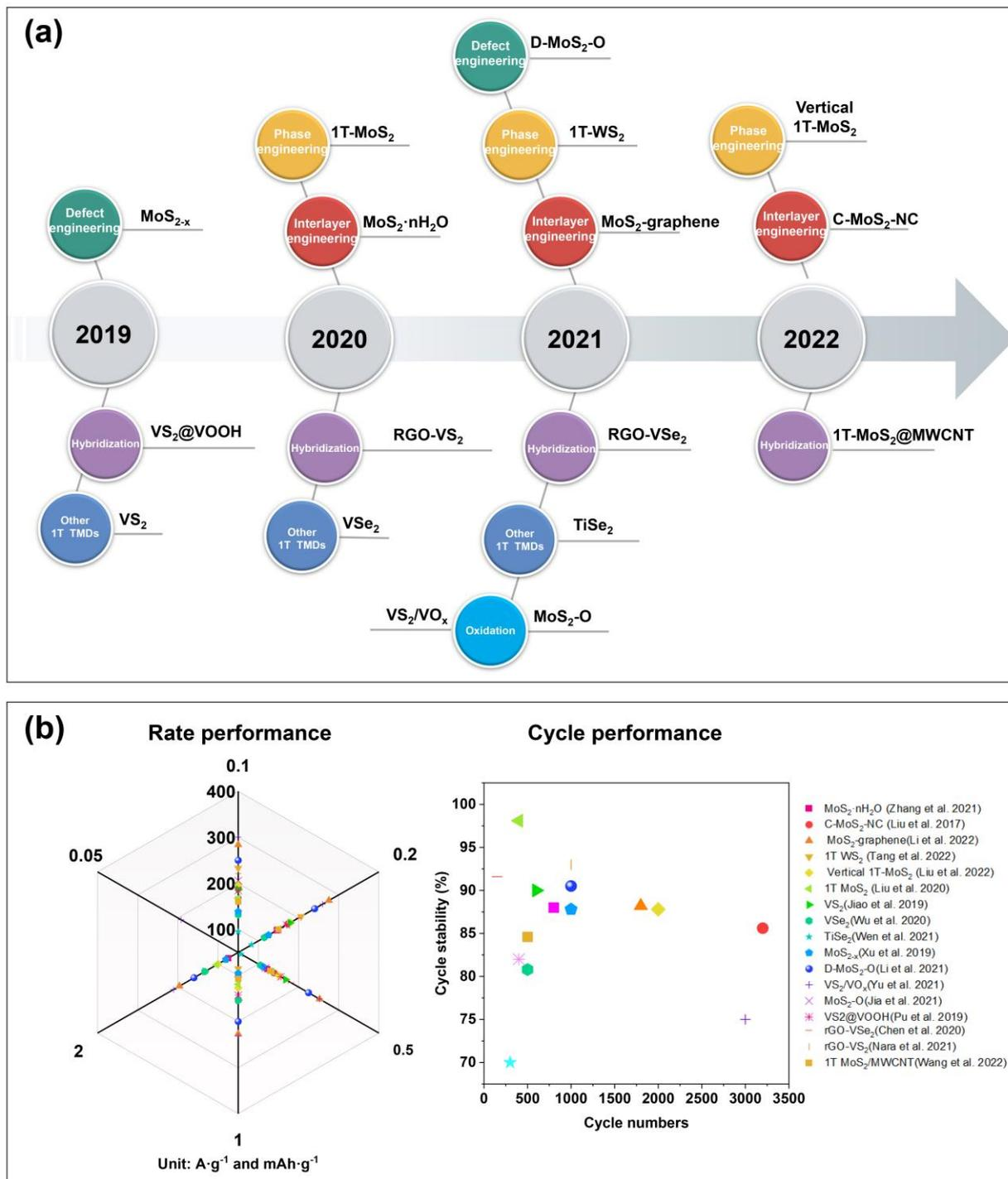
**Figure 8.** Summary of modified TMDs for high-performance ZIBs. (a) Timeline of developed strategies for TMD-based ZIB cathode. (b) The radar chart of the electrochemical performance of TMD materials as ZIB cathode. Refs. [12,14,16–18,22,23,28,29,42–44,47,51,54,55].
