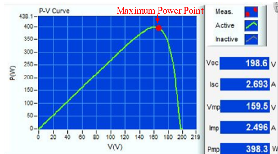
Figure 21. P-V characteristic curve of MPPT when the PVMA output power is at 400 W.
