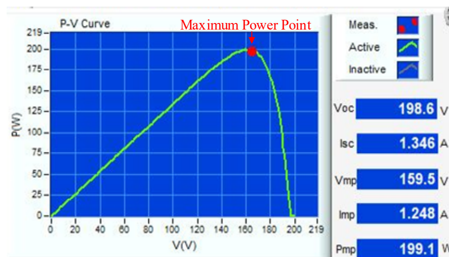
Figure 16. P-V characteristic curve of MPPT when the PVMA output power is at 200 W.
