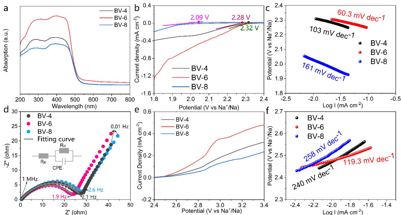
**Figure 2.** UV-visible absorption spectra (a), LSV curves for ORR at a scan rate of  $0.1 \text{ mV s}^{-1}$  (b), the corresponding Tafel slope for ORR (c), EIS (d), LSV curves for OER at a scan rate of  $0.1 \text{ mV s}^{-1}$  (e), and the corresponding Tafel slope for OER (f) of the  $\text{BiVO}_4/\text{CNTs}$  electrode under illumination.
