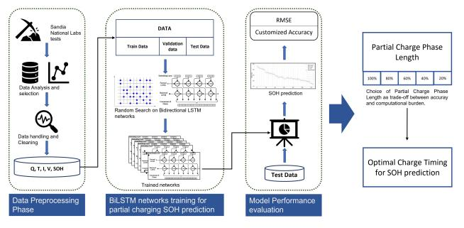
Figure 1. The proposed methodology for battery SOH prediction during partial charging processes.
