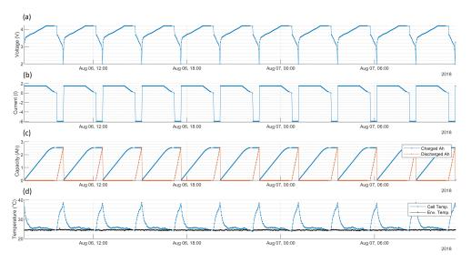
**Figure 2.** Example of constant current constant voltage charge profiles measured by Sandia National Laboratories during the performed experimental cell aging campaign. The cell operating parameters measured during the tests are (**a**) cell voltge (V), (**b**) current (A), (**c**) charged and discharged capacity (Ah), and (**d**) cell and environmental temperature (°C).
