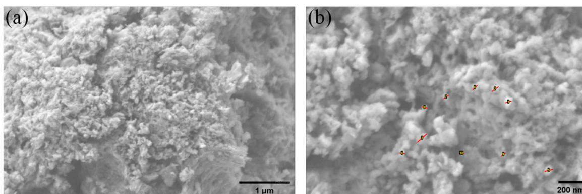
**Figure S1.** SEM image of TiHCF in different scales: (a) 1 μm and (b) 200 nm.
