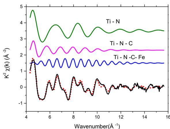
**Figure S2.** Details of the EXAFS analysis of the Ti K-edge of TiHCF, the comparison of the total theoretical signal (red) with the experimental one (black).
