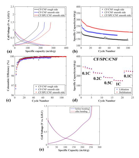
**Figure 5.** Electrochemical performance of the flexible CF negative electrodes: (**a**) the fourth charge/discharge voltage profiles cycled at 0.1 C; (**b**) specific capacity cycled at 0.1 C; (**c**) coulombic efficiency cycled at 0.1 C; (**d**) rate capabilities of the CF/SPC/CNF electrode; and (**e**) voltage profiles at 0.1 C before and after 4000 times of repeated bending.
