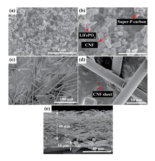
**Figure 4.** SEM images of the LFP-CF electrodes at different magnifications: (**a**,**b**) LFP layer surface morphology; (**c**,**d**) CF layer morphology; and (**e**) cross-sectional SEM image.
