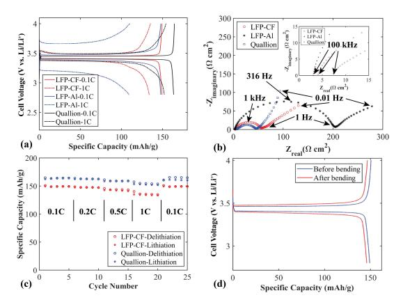
**Figure 6.** Electrochemical properties of electrodes: (**a**) charge/discharge voltage profiles of the LFP-CF, LFP-Al and Quallion electrodes cycled at 0.1 C and 1 C; (**b**) EIS of the LFP-CF, LFP-Al and Quallion electrodes; (**c**) rate capabilities of the LFP-CF and Quallion electrodes; and (**d**) voltage profiles at 0.1 C before and after 4000 times of repeated bending.
