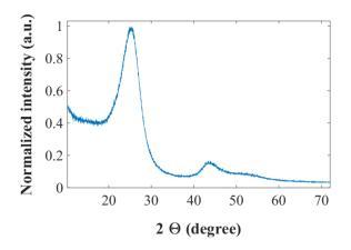
Figure 1. XRD spectrum for the Toho Tenax IMS65 CF.
