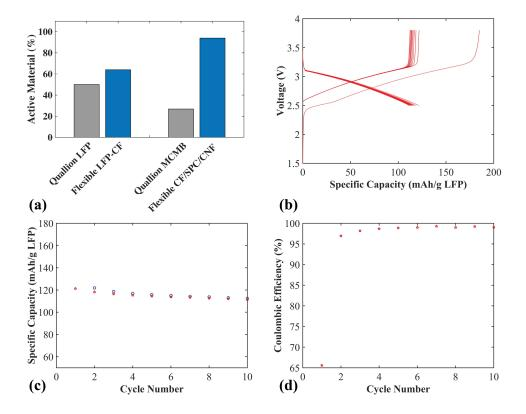
**Figure 7.** (a) Active material weight percentage of electrodes and current collector. Grey bars: Commercial Quallion LFP and MCMB electrodes. Blue bars: Flexible LFP-CF and CF/SPC/CNF electrode. Electrochemical performance of the LFP-CF versus CF/SPC/CNF electrodes cycled at 0.1 C: (b) voltage profiles; (c) specific capacity; and (d) coulombic efficiency.
