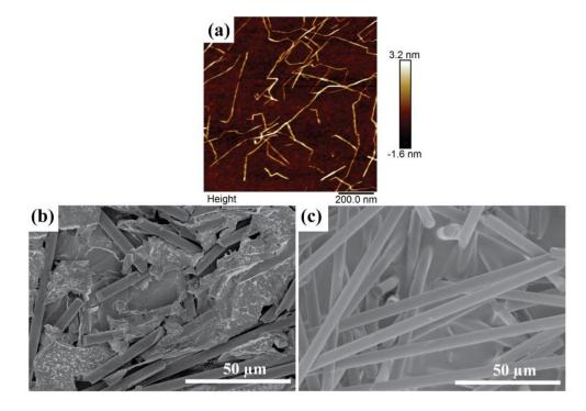
**Figure 2.** (a) AFM height image of CNF; SEM images of CF/CNF films from (b) smooth side; and (c) rough side.
