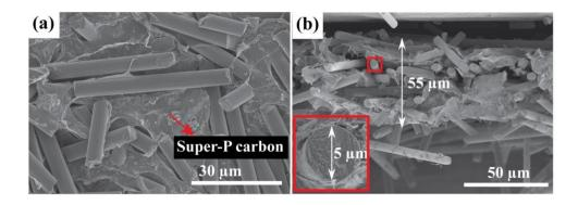
Figure 3. SEM images of CF/SPC/CNF films at (a) smooth surface side; and (b) cross-section.
