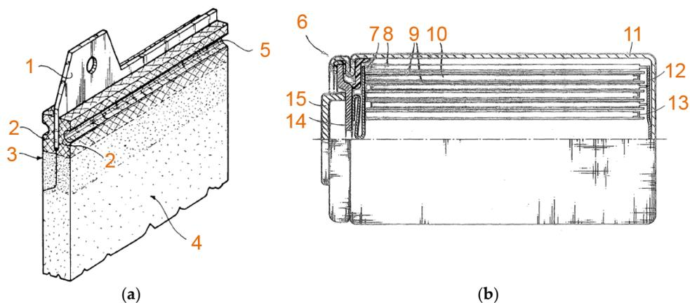
Figure 7. Schematics of (a) A metal-foam connection and (b) A cylindrical cell design from Alcatel. The parts are 1: metal strip, 2: foam without Ni(OH)<sub>2</sub>, 3: auxiliary foam, 4: main foam, 5: slot formed by compression [71]; 6: folded part of can, 7: metal tab, 8: negative electrode, 9: separator, 10: positive electrode, 11: can, 12: a piece of nickel plated steel disc, 13: adhesive tape, 14: lug, and 15: cover [72].
