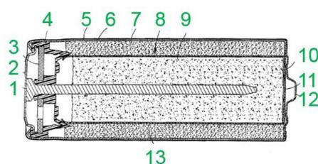
**Figure 10.** Schematic of a cylindrical cell design from Eveready/Freudenberg. The parts are 1: negative current collector, 2: negative terminal, 3: metal plate, 4: polymer seal, 5: metalized plastic film, 6: steel can, 7: tubular positive electrode, 8: separator, 9: negative electrode, 10: bottom of negative electrode, 11: bottom of folding cylinder, 12: positive terminal, and 13: folding can [118].
