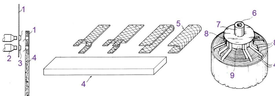
**Figure 2.** Schematics of three different designs of current collectors by SAFT. The parts are 1: metal plate, 2: plug, 3: indent, 4: electrode [37]; 5: expanded metal or perforated metal strip [38]; 6: threaded holes, 7: terminal assembly, 8: conducting strip, and 9: shoulder [40].
