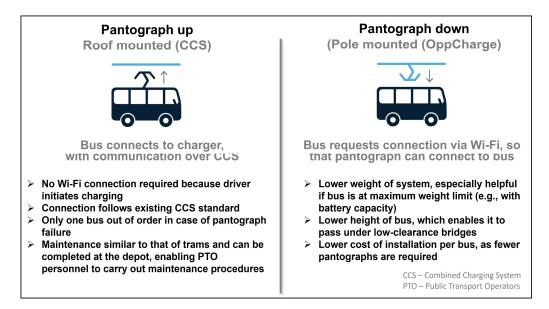
Figure 7. Figure illustrating the benefits of each pantograph system. Adapted from [62].
