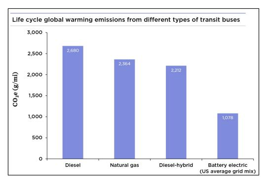
Figure 9. CO<sub>2</sub> emissions from buses. Reproduced with permission from [81].
