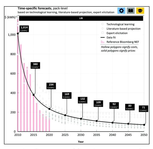
Figure 4. Prediction of battery prices over time [53]. Copyright 2021, Energy & Environmental Science.
