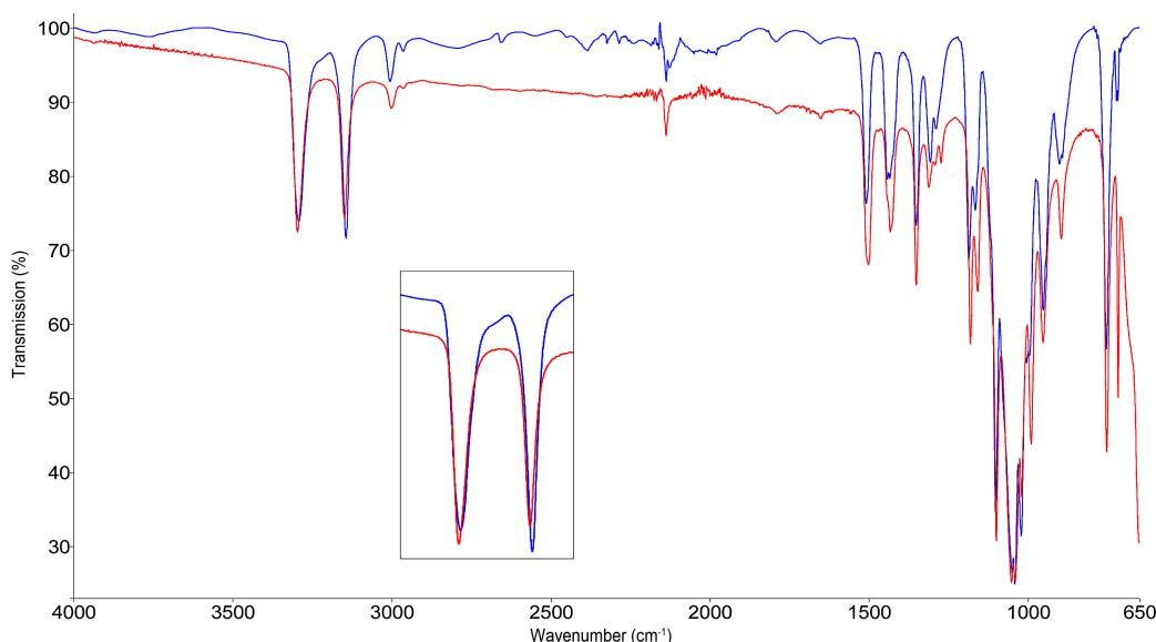
**Figure 4.** Variable temperature mid-infrared spectra of **1**, high-spin state at 300 K (red) and partial low-spin state at 100 K (blue).
