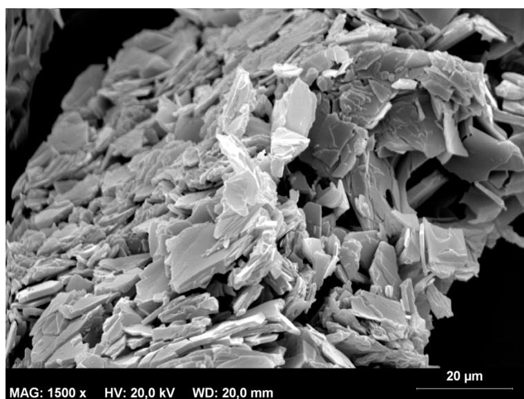
**Figure 2.** SEM picture of  $[\text{Fe}(\text{prgTz})_6](\text{BF}_4)_2$  at 298 K, magnification 1500 times.
