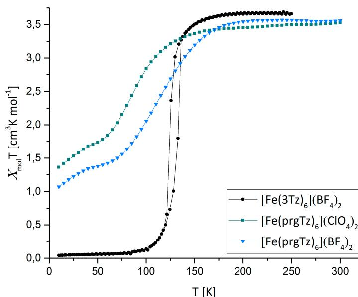
**Figure 1.** Temperature dependence of  $\chi_{\text{mol}}T$  for **1** (blue), **2** (green) and  $[\text{Fe}(\text{3tz})_6](\text{BF}_4)_2$  (black) [26,27].
