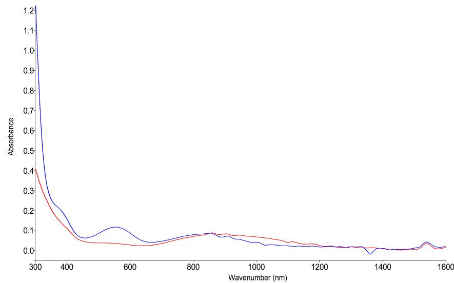
**Figure 6.** Variable temperature visible/near-infrared spectra of **1**, HS state at 300 K (red) and partial LS state at 130 K (blue).
