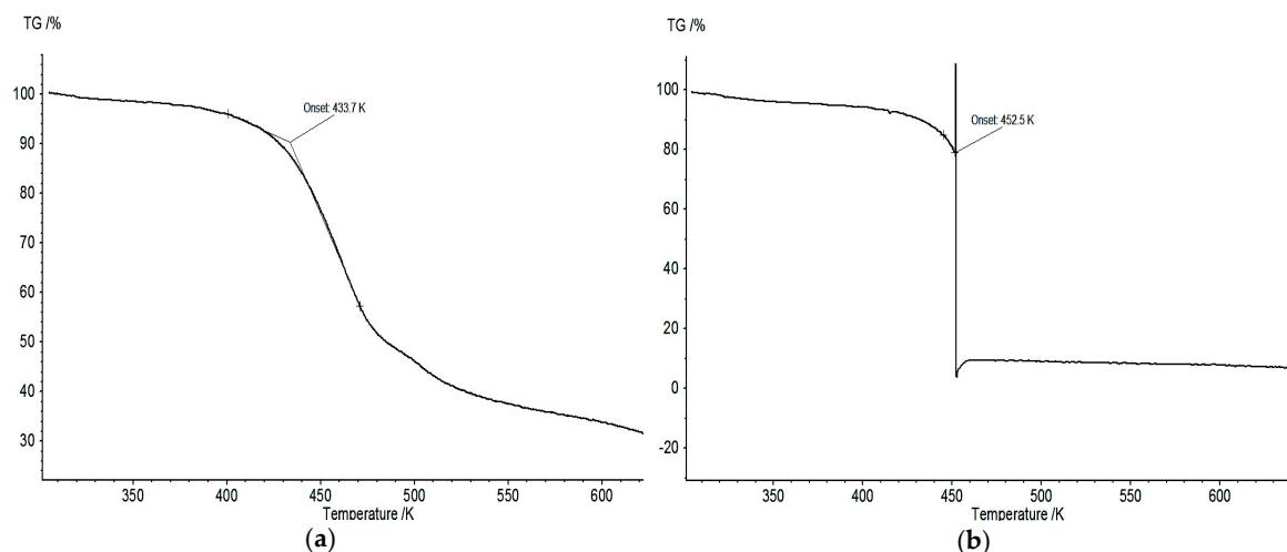
**Figure 7.** (a) Thermogravimetric analysis of  $\text{BF}_4$ -complex **1**; and (b) TGA curve of  $\text{ClO}_4$ -complex **2**.
