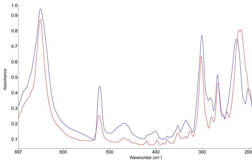
**Figure 5.** Variable temperature far-infrared spectra of **1**, HS state at 300 K (red) and partial LS state at 100 K (blue).
