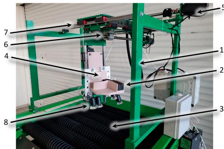
**Figure 1.** The setup for the hyperspectral imaging of apple fruits. Designations: chassis (1); the hyperspectral camera (2), a table with rubber rollers (3) camera suspension (4), stepper motors (5, 6) and the transmission (7), light source (8).
