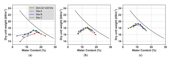
**Figure 5.** Compaction curves with compaction types of (**a**) A<sub>0</sub>, (**b**) A, and (**c**) C for soil samples from Sites A, B, and C.
