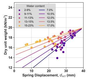
**Figure 11.** Relationship of dry unit weight to spring displacement dependent on water content. Correlation models are shown as solid lines.
