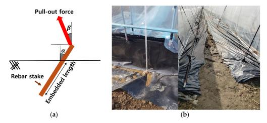
**Figure 16.** (a) Description of inclination angles of installation ( $\alpha$ ) and pull-out direction ( $\beta$ ) and (b) photos of field installation conditions.
