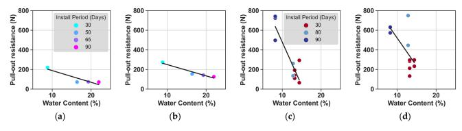
**Figure 15.** Ultimate pull-out resistance of rebar stakes with different embedded lengths versus variation of water contents over time. Site A with human weight compaction, (**a**) 20 cm depth, and (**b**) 40 cm depth. Sites B and C with natural compaction, (**c**) 20 cm depth, and (**d**) 40 cm depth.
