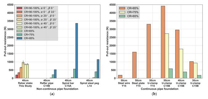
U-clamp method at a 40 cm embedment depth reaching an  $R_{pull-out}$  of 2953 N. This  $R_{pull-out}$  is also about three times that of rebar stakes.
