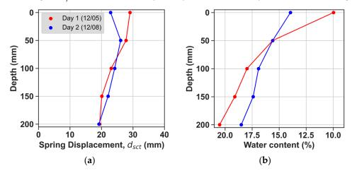
Figure 17. Variation in (a) spring displacement and (b) water content at Site A.
