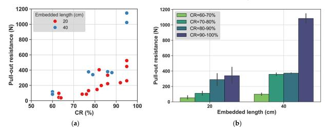
**Figure 13.** Ultimate pull-out resistance of rebar stakes with varying compaction rates and embedded lengths. (a) Scatter plot for pull-out resistance versus compaction rate and (b) bar chart for pull-out resistance versus embedded length.
