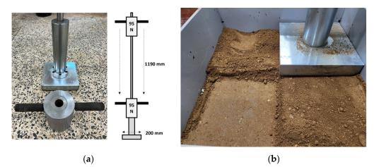
Figure 8. Photos of soil box test: (a) compaction rammer [32] and (b) soil box.
