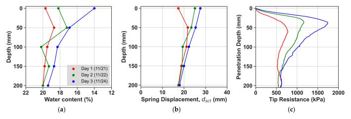
**Figure 12.** (a) Water content, (b) spring displacement of soil compaction meter, and (c) tip resistance of cone penetration test, showing the variations at each depth according to climatic changes at Site A.
