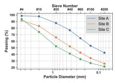
**Figure 4.** Grain size distributions of samples from the source site (Site A) and field test sites (Sites B and C).
