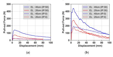
**Figure 14.** Pull-out resistance with different installation period (IP) and embedment depth (ED) at Site A by different compaction levels: (**a**) human weight and (**b**) compactor.
