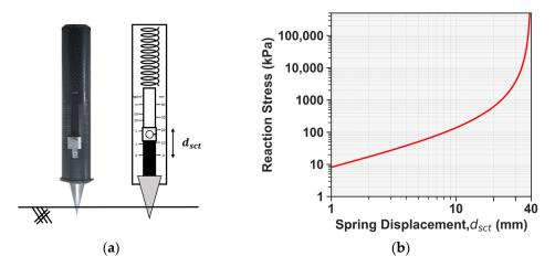
Figure 6. Soil compaction meter. (a) Photo [32]; (b) spring displacement versus soil reaction stress.
