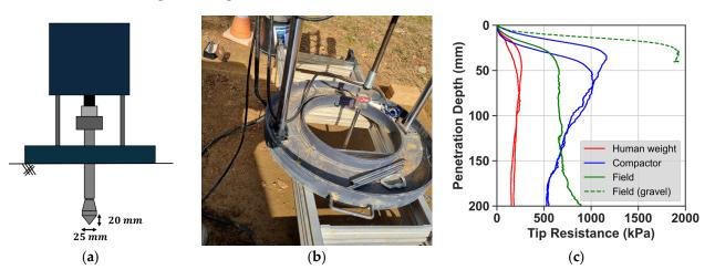
**Figure 10.** (a) Schematic drawing and (b) photo of portable cone penetrometer developed in this study. (c) Tip resistances at Site A with varying field compaction levels (human weight and compactor) and at Site B (field).
