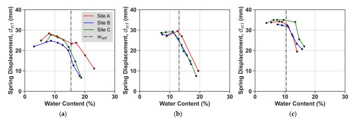
**Figure 7.** Spring displacement ( $d_{sct}$ ) of soil compaction meter versus water content for soil samples from compaction types of (**a**) A<sub>0</sub>, (**b**) A, and (**c**) C.
