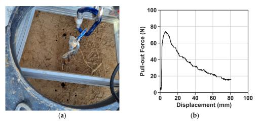
**Figure 9.** Rebar stake pull-out test. (**a**) Photo; (**b**) example of the measurement of pull-out force versus pull-out displacement.
