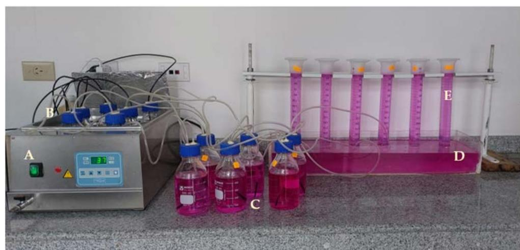
**Figure 1.** The experimental facility used in the research. (A) Thermostated water-bath with recirculation. (B) Anaerobic digester flasks. (C) Bubbling traps for  $\text{CO}_2$  capture. (D) Immersion cuvette. (E) Inverted test tubes for methane measurement.
