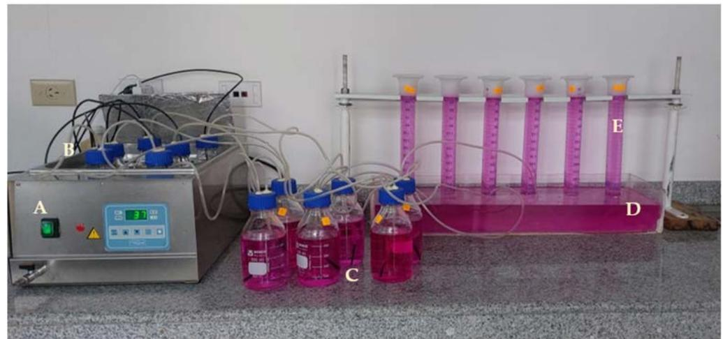
**Figure 1.** The experimental facility used in the research. (A) Thermostated water-bath with recirculation. (B) Anaerobic digester flasks. (C) Bubbling traps for CO<sub>2</sub> capture. (D) Immersion cuvette. (E) Inverted test tubes for methane measurement.
