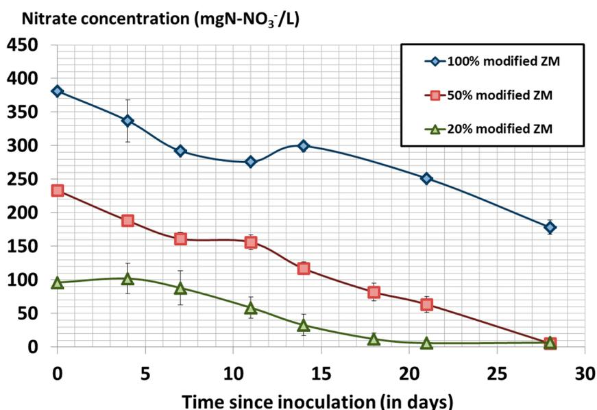
Figure 5. Nitrate concentrations in mgN-NO<sub>3</sub><sup>-</sup>/Lin 100% (blue diamonds), 50% (red squares), and 20% (green triangles) modified ZM growing Spirulina, triplicates.
