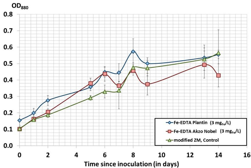
**Figure 6.** OD<sub>880</sub> measurements of Spirulina grown using Fe-EDTA from Plantin at 3 mg<sub>Fe</sub>/L (blue diamonds), Fe-EDTA from Akzo-Nobel at 3 mg<sub>Fe</sub>/L (red squares) and modified ZM (control, 2 mg<sub>Fe</sub>/L in the form of FeSO<sub>4</sub>·6H<sub>2</sub>O with 50 mg/L of EDTA, green triangles), in duplicate. Error bars are standard deviations of the biological duplicates.
