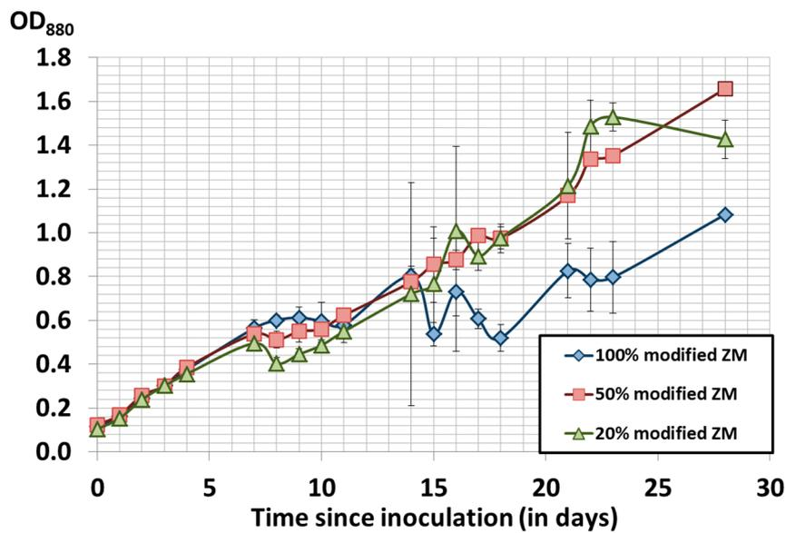
**Figure 3.** OD<sub>880</sub> measurements of Spirulina grown in 100% (blue diamonds), 50% (red squares), and 20% (green triangles) modified ZM, triplicates. Error bars are standard deviations of the biological triplicates.
