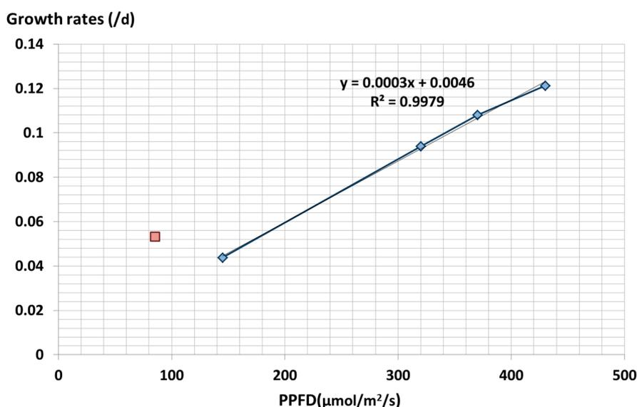
**Figure 8.** Spirulina growth rates with respect to PPF. The correlation (blue diamonds) does not include the first point at 85 μmol/m<sup>2</sup>/s (red square). No replicate.
