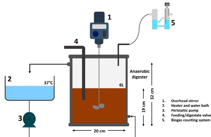
**Figure 1.** Schematic representation of the laboratory-scale anaerobic digesters.
