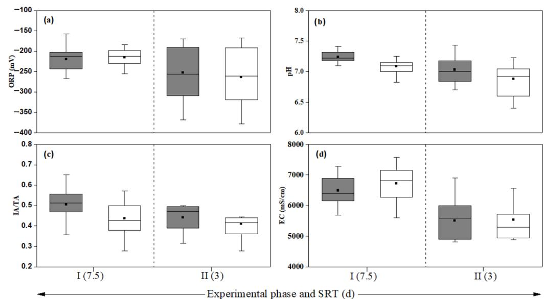
**Figure 2.** Conditions of operational parameters of: (a) ORP, (b) pH, (c) alkalinity ratio IA/TA, and (d) EC. For the control reactor (■) and reactor with pretreatment (□) at SRTs (solids retention times) of 7.5 and 3 days.
