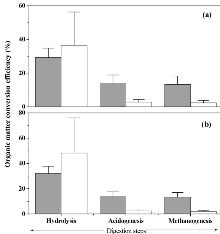
**Figure 4.** Organic matter conversion efficiency in the different anaerobic digestion stages in the control reactor (CR) (a) and the reactor with pretreatment (PTR) (b) at SRTs (solids retention times) of 7.5 (■) and 3 days (□).
