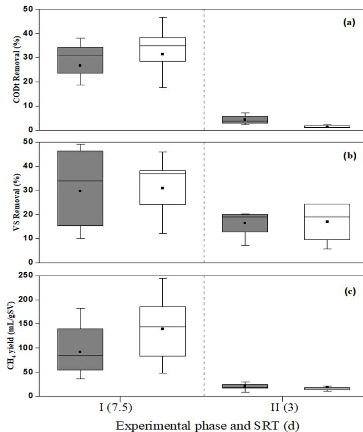
**Figure 3.** Boxplot summarizing the operational performance of the reactors, expressed in terms of their removal efficiencies and methane yields. (a)  $\text{COD}_t$ , (b) VS, and (c)  $\text{CH}_4$  production. Control reactor (■) and reactor with pretreatment (□).
