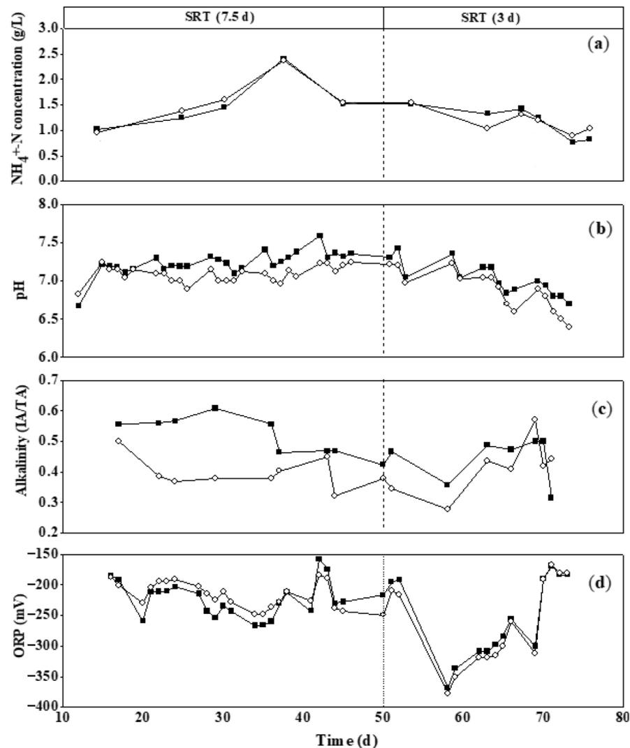
**Figure 5.** Behavior of the monitored operational parameters: (a)  $\text{NH}_4^+\text{-N}$ , (b) pH, (c) alkalinity ratio (IA/TA), and (d) ORP. Data for the control reactor (■) and reactor with pretreatment (□) at solids retention times of 7.5 and 3 days.
