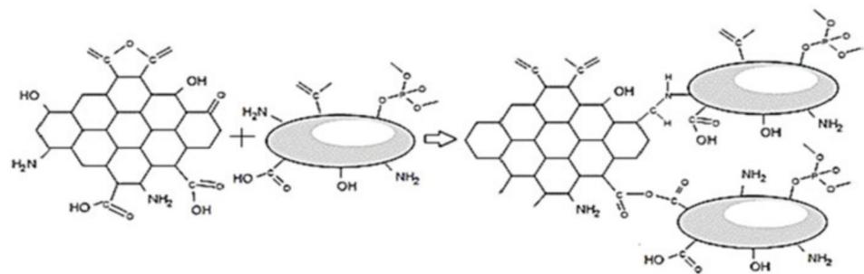
**Figure 13.** The formation of covalent bonds between the surfaces of microbial cells and the carbonized materials considerably contributes to the stability of the biocomposite materials. Reprinted with permission from Ref. [50]. Copyright 2020, Jenny Stanford Publishing Pte. Ltd.
