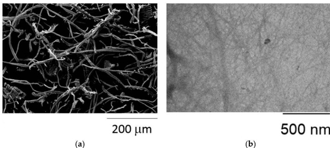
**Figure 4.** (a) Micrograph obtained using SEM of rice husk treated with NaOH followed by peracetic acid, and (b) micrographs obtained using TEM of the cellulose nanofibers from rice husk (extraction at 2 h). Reprinted with permission from Ref. [24]. Copyright 2016, Materials Research.
