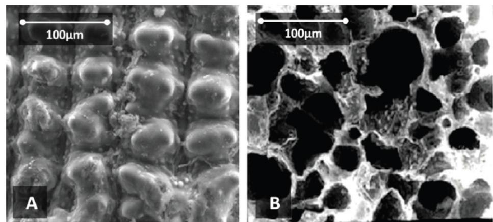
**Figure 12.** Electron microscopic images of rice shells in native state (A) and after carbonization at 650 °C (B). Reprinted with permission from Ref. [50]. Copyright 2020, Jenny Stanford Publishing Pte. Ltd.
