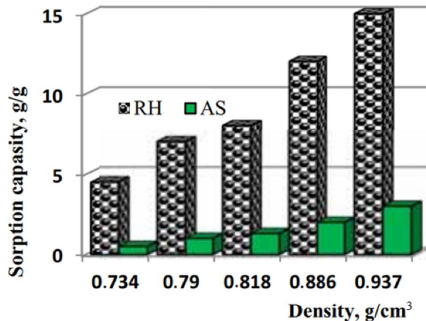
**Figure 3.** Sorption characteristics of carbonized rice husk and carbonized apricot stone as a function of petroleum product density. Reprinted with permission from Ref. [22]. Copyright 2014, Ministry of Education and Science of the Republic of Kazakhstan.
