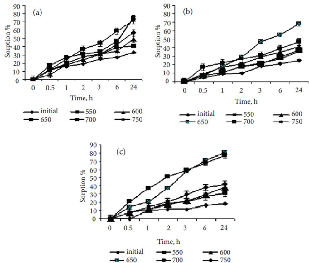
**Figure 16.** Dynamics of sorption of *Rhodotorula glutinis* var. *glutinis* (a), *Pseudomonas mendocina* (b) and *Pseudomonas aeruginosa* (c) cells onto the surface of initial and carbonized AS. Reprinted with permission from Ref. [50]. Copyright 2020, Jenny Stanford Publishing Pte. Ltd.
