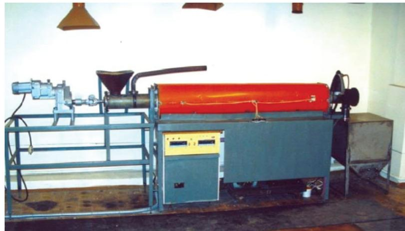
**Figure 10.** Pilot setup for flame carbonization of diverse raw plant materials. Reprinted with permission from Ref. [45]. Copyright 2012, IntechOpen.
