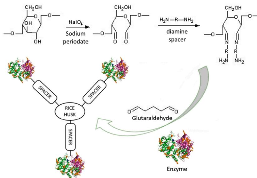
**Figure 1.** Schematic illustration of the oxidation and functionalization of the cellulosic fraction of RH for the covalent immobilization of Lipase B from *Candida Antarctica*. Reprinted with permission from Ref. [10]. Copyright 2018, MDPI.
