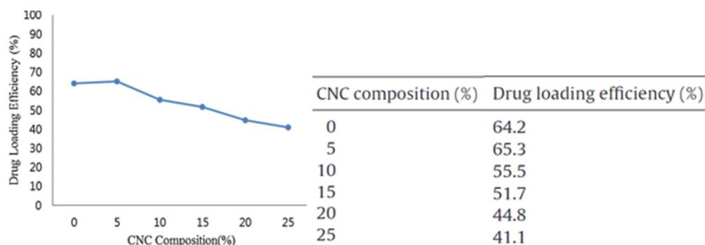
**Figure 7.** Drug-loading efficiency of cellulose nanocrystal–gelatin hydrogels and drug-loading efficiency data for gelatin hydrogels and CNC gelatin hydrogels reinforced with different amounts of CNC. Reprinted with permission from Ref. [41]. Copyright 2016, Elsevier.
