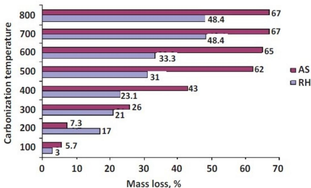
**Figure 11.** Dynamics of change in the mass of RH and AS in the carbonization process at various temperatures. Reprinted with permission from Ref. [50]. Copyright 2020, Jenny Stanford Publishing Pte. Ltd.
