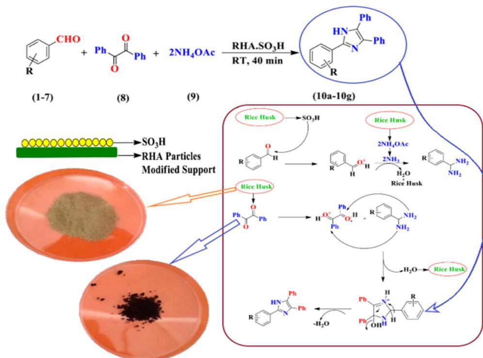
**Figure 5.** Scheme for the synthesis of Imidazole with RH ash. Reprinted with permission from Ref. [30]. Copyright 2022, Elsevier.
