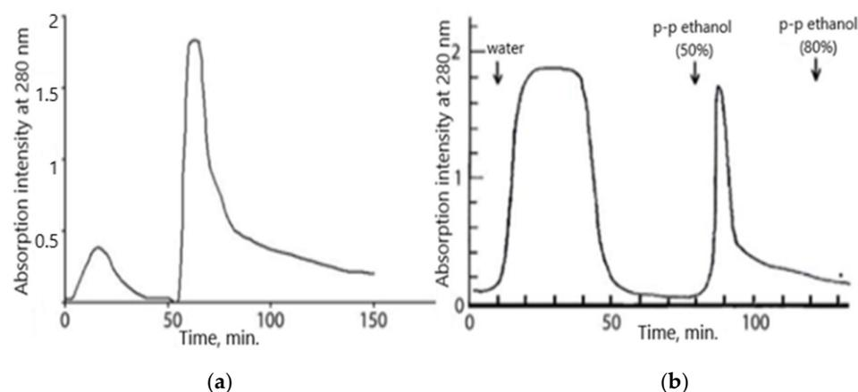
**Figure 2.** Fusicoccin chromatographic separation curves on column with carbonized RH (a) and octylsepharose 4B-CL organic gel (b). Reprinted with permission from Ref. [14]. Copyright 2007, KazNU.
