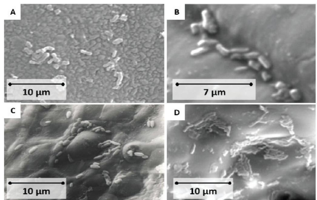
**Figure 14.** Subsequent stages of colonization of NCSs by *Lactobacilli*. (A) Carbonized rice husk, initial adsorption; (B) carbonized grape stones, initial adsorption; (C,D) carbonized grape stones and micro-colony formation (respectively). Reprinted with permission from Ref. [50]. Copyright 2020, Jenny Stanford Publishing Pte. Ltd.
