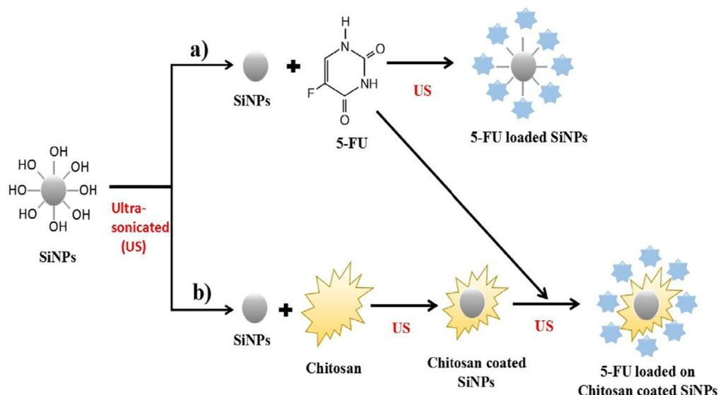
**Figure 6.** Schematic of the functionalization of 5-FU on SiNPs by (a) Direct conjugation (SiNPs conjugated with 5-FU) and (b) indirect conjugation (chitosan-coated SiNPs conjugated with 5-FU). Reprinted with permission from Ref. [31]. Copyright 2020, Elsevier.
