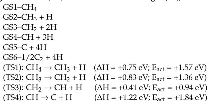
In the gas phase, the activation barriers for CH<sub>4</sub> decomposition are substantially larger than on the surface of the copper substrate. All the reactions are endothermic except for the formation of carbon. The entire reaction is described as follows:
