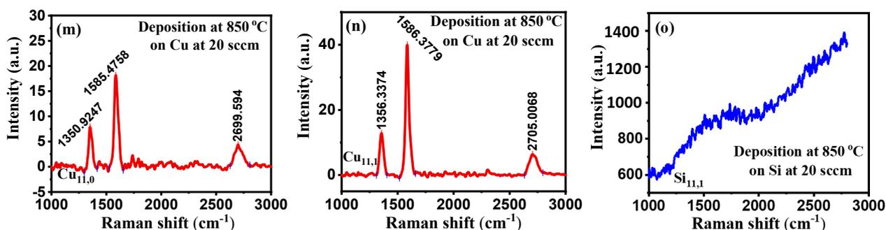
**Figure 4.** (a–o) Raman spectra at constant  $\text{CH}_4$  flow rate at 20 sccm with different deposition temperatures on Cu and Si substrates.
