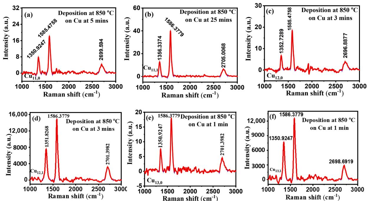
**Figure 5.** (a–f) Raman spectra at different deposition times with a constant CH<sub>4</sub> flow rate of 20 sccm and 850 °C deposition temperature.
