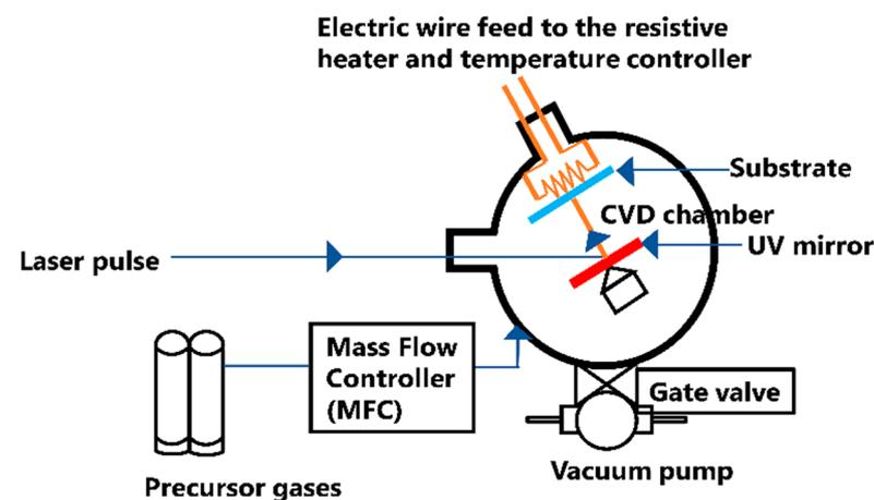
**Figure 1.** Schematic diagram of the deposition process in the chamber.
