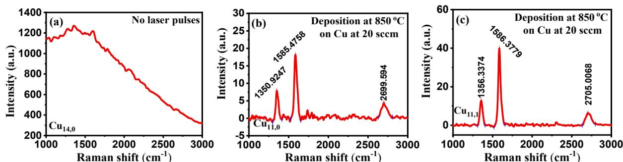
**Figure 6.** (a–c) Raman data plots showing the effect of: (a) no laser pulses; (b) laser incident spot; (c) laser non-incident spot on PyC deposition.
