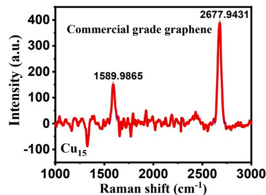
Figure 2. Raman spectra of pristine high-quality graphene.
