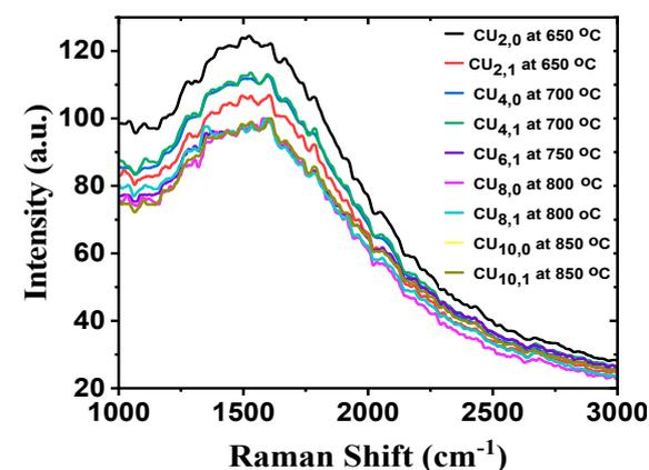
Figure 3. Raman spectra at a constant  $\text{CH}_4$  flow rate at 10 sccm and different deposition temperatures.
