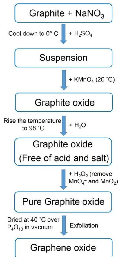
**Figure 6.** Schematic diagram showing Hummers method [31].
