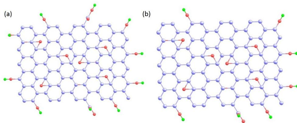
**Figure 2.** Structures of (a) graphene oxide and (b) reduced graphene oxide [light purple-carbon, red-oxygen and green-hydrogen].
