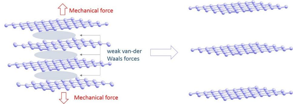
**Figure 4.** Mechanical exfoliation process in graphite.
