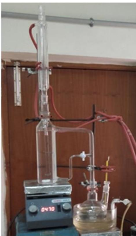
Figure S2. A digital photograph showing the continuous liquid-liquid extraction apparatus employed for separating bmim[BF<sub>4</sub>] RTIL from NaBr salt from the reaction mixture solution.
