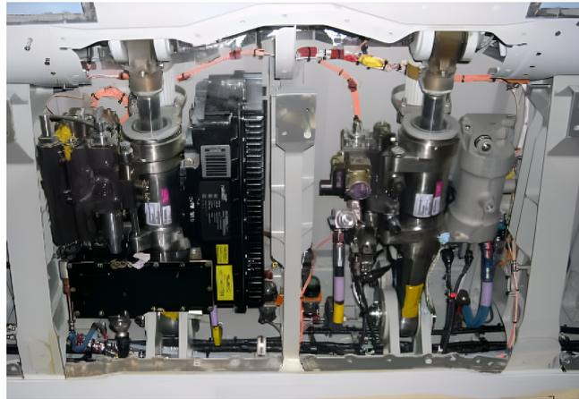
**Figure 2.** Comparison of installed aileron EHA (left) and conventional hydraulic actuator (right) [9].
