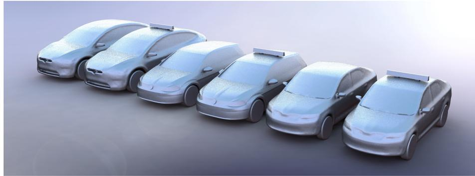
Figure 5. Rendered image of the three additional taxi types, crossover, hatchback, and notchback.
