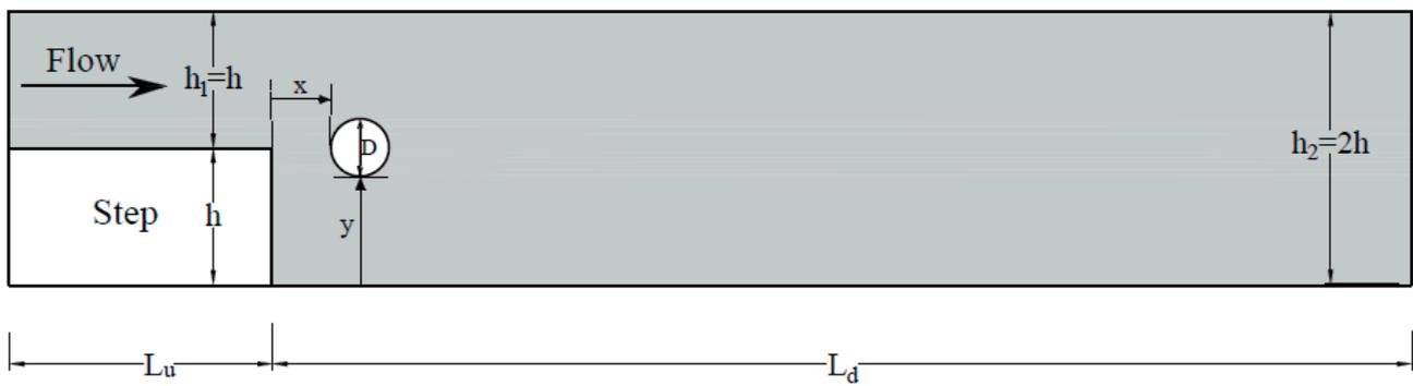
Figure 1. Schema of BFSF with a cylinder in laminar flow simulations (BFSF 2) (not to scale).
