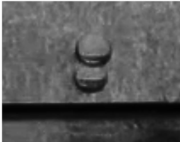
**Figure 14.** 5 mm water drops settling in oil stuck together without coalescing.
