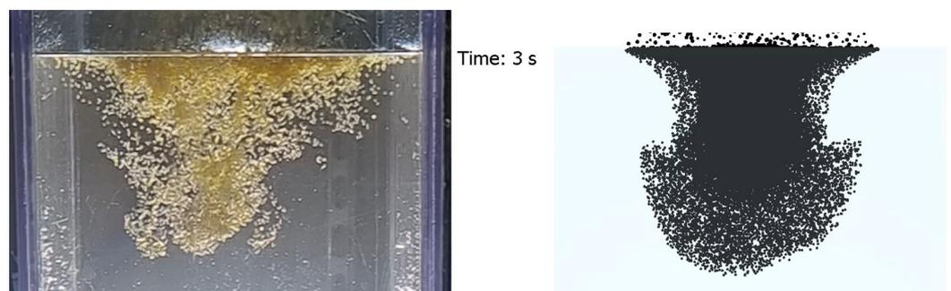
**Figure 13.** Comparison of the start of the channeling phenomenon in experimental and simulated setups.
