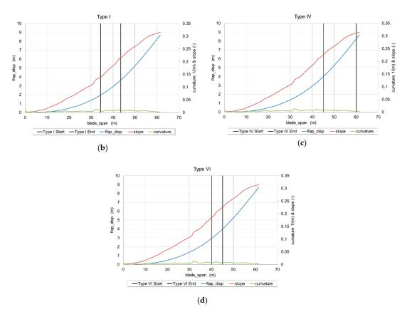
**Figure 2.** (a) Flap deflection, slope, and curvature of the first eigenmode of the considered wind turbine (WT) blade, (b) location of tip accumulator of type I, (c) location of tip accumulators of type IV, and (d) location of tip accumulators of type VI.
