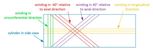
**Figure 7.** Qualitative illustration of the different winding directions that can be applied in the manufacturing process of a carbon fibre-reinforced plastic (CFRP) cylinder (the angles are only examples for illustrating the concept).
