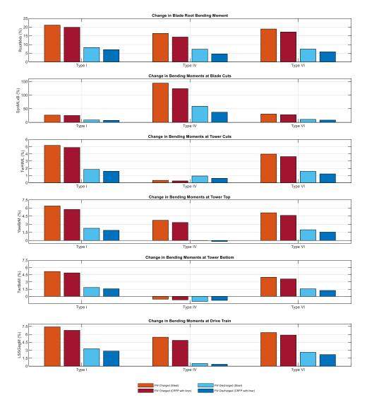
**Figure 12.** Comparison of changes in fatigue loads in (from top to bottom) blade root bending moment, bending moments at blade cuts, bending moments at tower top, bending moments at tower bottom, and bending moments at drive train, between steel accumulator and CFRP with metal liner accumulator for FW types I, IV, and VI in charged (red) and discharged (blue) status, both with respect to the ultimate loads of the original WT without FW system.
