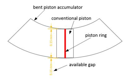
Figure 5. Illustration of a bent piston accumulator in the side view (not to scale).
