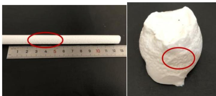
**Figure 3.** Pores appearing in gel.
