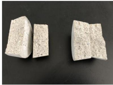
**Figure 19.** Fractured impermeability test specimens.
