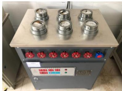
**Figure 21.** Impermeability tester.
