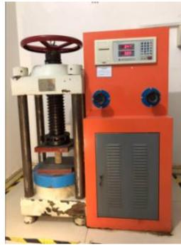
**Figure 17.** Electrohydraulic pressure testing machine.
