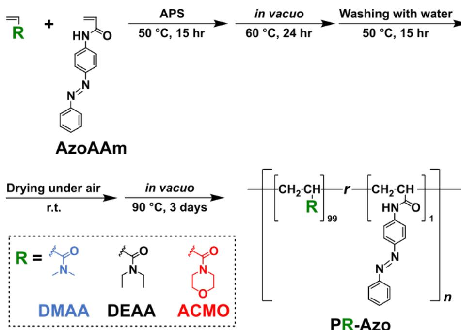
**Figure 1.** Chemical structures of the moisture-sensitive photoresponsive hydrogels (PDMAA-Azo, PDEAA-Azo, and PACMO-Azo) and details of the polymerization and posttreatment. The hydrogels were prepared in the bulk state. Namely, liquid monomers served as the solvent as well as monomers.
