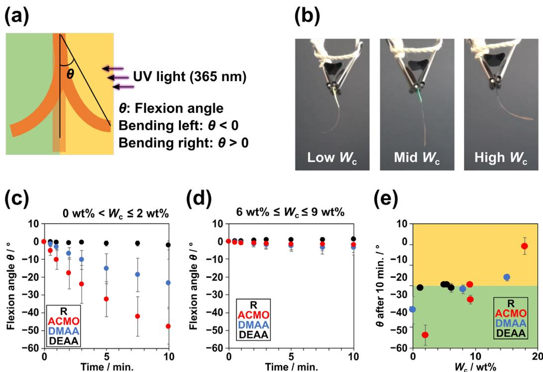
**Figure 2.** (a) Illustration defining the flexion angle  $\theta$  and the positive and negative bending directions. (b) Snapshots of PACMO-Azo with three different water contents ( $W_c$ ) at 8 min. Time dependencies of the flexion angles of PR-Azo with (c) low  $W_c$  (0–2 wt%) and (d) mid  $W_c$  (6–9 wt%); (e)  $\theta$  of PR-Azo after UV light irradiation for 10 min with various  $W_c$  values.
