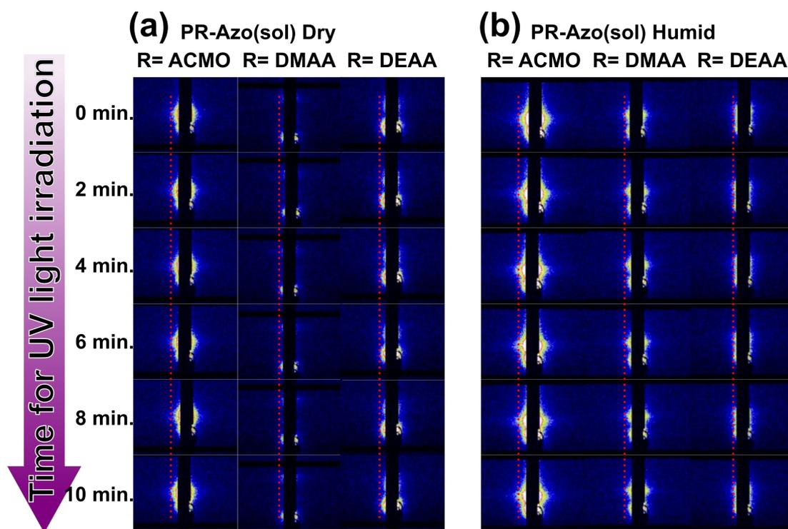
**Figure 3.** Time dependencies of 2D GISAXS scattering patterns of PR-Azo(sol) in (a) the dried states and (b) humid states during UV light irradiation.
