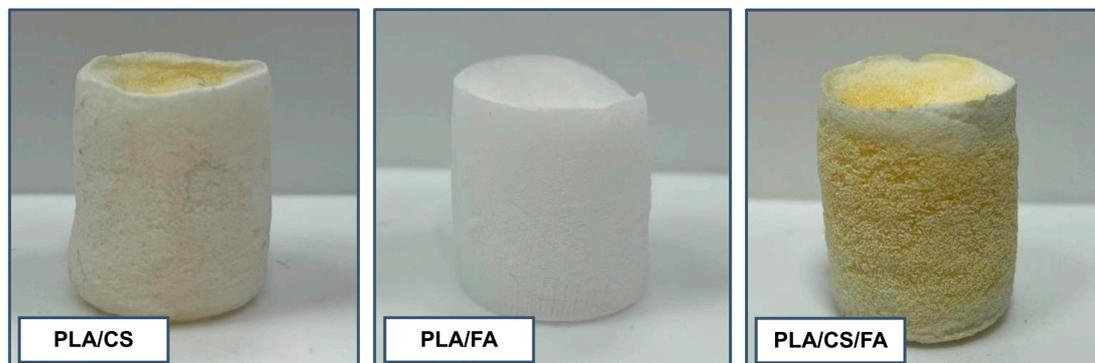
**Figure 1.** Visual comparison between polylactide scaffolds differing in surface modification type.
