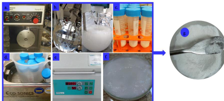
**Figure 6.** Graphical summary of the synthesis procedure of calcium-polyphosphate (CaPP) particles employing the coprecipitation method: (a) flow pump; (b) controlled addition of CaCl<sub>2</sub>·2H<sub>2</sub>O solution (1 mL/min; pH = 10) into the NaPP solution; (c) After 4 h of stirring, distribution of the crude product in falcon tubes; (d) washing of CaPP (twice with water and twice with ethanol); (e) Centrifugation after every wash; (f) CaPP slurry obtained; (g) CaPP dried fine powder.
