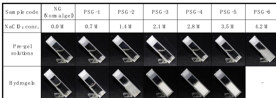
**Figure 2.** Photographs of pre-gel solutions and hydrogels in different conditions of polymerization.
