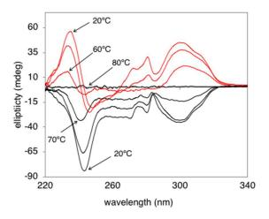
**Figure 2.** ICD spectra of 1.5% (w/w) BBO8-Me n-octanol gel-sol transitions (Cycle 1, increasing temperature, black) and sol-gel (Cycle 2, decreasing temperature, red).
