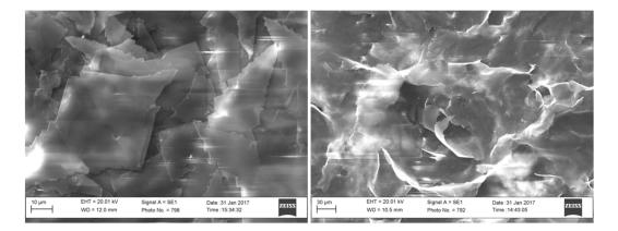
**Figure 5.** SEM images of BBO6-Me (left) and BBO10-Me (right) xerogels obtained from 1.5% in n-octanol gels.
