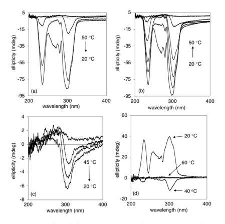
**Figure 3.** Hysteresis study of 1.5% (w/w) BBO8-Et n-octanol gel. (**a**) Sol-gel, Cycle 1; (**b**) gel-sol, Cycle 2; (**c**) sol-gel, Cycle 3; (**d**) sol-gel, Cycle 4.
