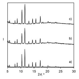
**Figure 9.** XRD diffractograms ( $\lambda = 1.5418$  Å) of BBO8-Me xerogels obtained from gels prepared in (**a**) n-octanol, (**b**) n-butanol and (**c**) ethanol.
