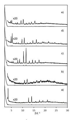
**Figure 8.** XRD diffractograms ( $\lambda = 1.5418$  Å) obtained for xerogels. (**a**) BBO6-Me; (**b**) BBO8-Me; (**c**) BBO8-Et; (**d**) BBO10-Me; (**e**) BBO10-Et.
