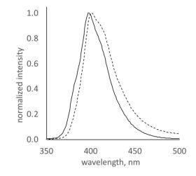
**Figure 1.** Normalized emission spectra of BBO8-Me in  $10^{-5}$  M n-octanol solution (solid) and 1.5% (w/w) n-octanol gel (dashed) excited at 270 nm.
