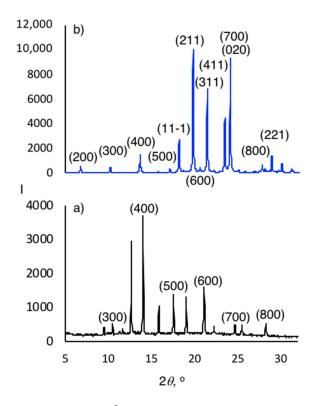
**Figure 7.** XRD diffractograms ( $\lambda$  = 1.5418 Å): (**a**) BBO6-Me xerogel; (**b**) simulated BBO6-Me based on single-crystal X-ray diffraction results.
