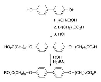
**Scheme 1.** Synthesis of biphenyl gelators. BBO6-Me (n = 5, R = Me), BBO6-Et (n = 5, R = Et), BBO8-Me (n = 7, R = Me), BBO8-Et (n = 7, R = Et), BBO10-Me (n = 9, R = Me), BBO10-Et (n = 9, R = Et).
