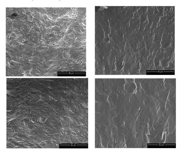
**Figure 5.** Cryo-SEM micrographs of 6% "intact" (**on the left**) and pre-sheared gels (**on the right**). Micrographs at different magnifications: 40 and 20 µm (from **top** to the **bottom**).
