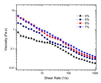
**Figure 3.** Viscosity (mean) as a function of shear rate for 4%, 5%, 6%, and 7% gels. These curves describe the flow behavior of the sheared and time independent fluid. The Extended Herschel-Bulkley model was applied to describe the flow characteristics of the gels. Measurements were carried out in triplicate. Error bars shown in the plot were calculated using a 95% confidence interval determined with the software OriginPro 2016 (OriginLab Corporation, Northampton, MA, USA).
