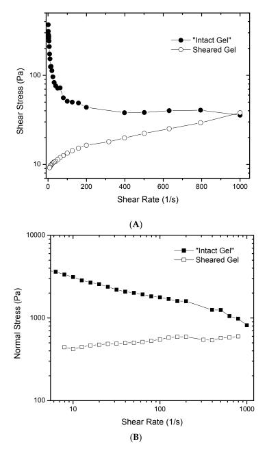
**Figure 4.** "Intact" and sheared gels: (**A**) shear stress versus shear rate of 6% gels. A typical curve of shear thinning fluid is only observed for the sheared gel (empty circle marks); (**B**) first normal stress versus shear rate of 6% gels. Filled squares show the decrease in normal stress of the "intact" gel at different shear rates. Empty squares show no variation of normal stress at different shear rates.
