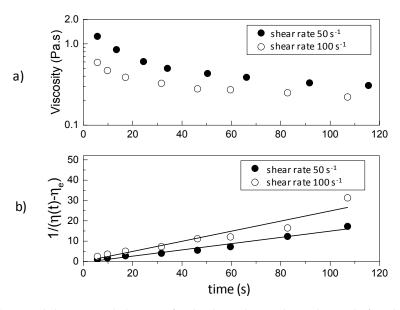
**Figure 1.** (a) Typical thixotropic behavior of a rheological time dependent gel after the application of constant shear rates of 50 1/s and 100 1/s; (b) schematic of the approach used to determine the parameters defining the structural parameter  $\lambda(\dot{\gamma}, t)$  from Equation (10). Data used are from a 5% silica gel.
