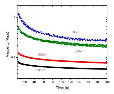
**Figure 6.** Viscosity of 4% "intact" gel as a function of time at different constant shear rates (50, 100, 500, and  $1000 \text{ s}^{-1}$ ).
