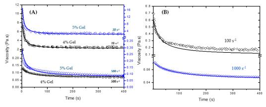
**Figure 7.** (**A**) Experimental (symbols) and predicted viscosity (lines) data for 4% and 5% gels at 10 and 500 s<sup>-1</sup>. The 4% data is plotted in the left *Y*-axis and is represented by square symbols. The 5% data is plotted in the right Y-axis and is represented by diamond symbols; (**B**) calculated viscosity assuming  $\lambda_e = 1$  for 4% gels at shear rates of 100 and 1000 s<sup>-1</sup>.
