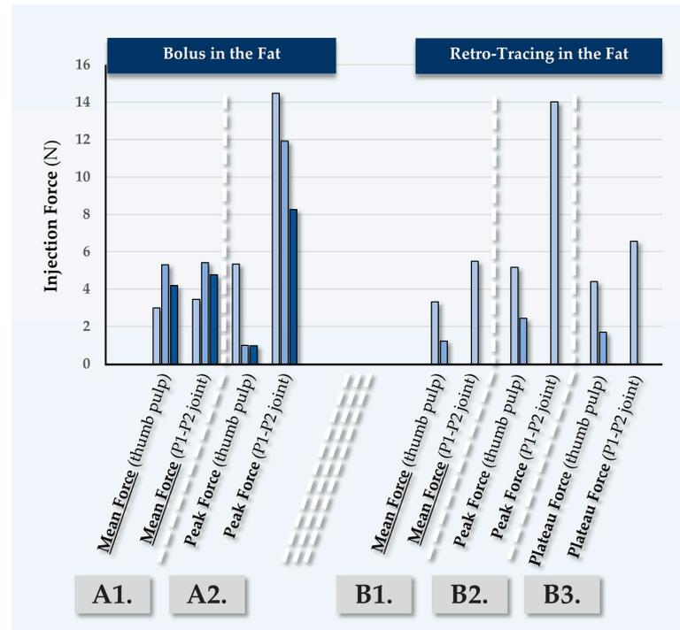
**Figure 7.** Quantitative results of in vivo dermal filler product injectability evaluation in Participant N°3, using the MaiLi® Volume dermal filler. Mean forces (A1) and peak forces (A2) were plotted for bolus injections in the fat. Mean forces (B1), peak forces (B2), and plateau forces (B3) were plotted for retro-tracing injections in the fat. Selected injection force data and injection force profiles are presented in Figure S10 and in Table S3. N, Newtons.
