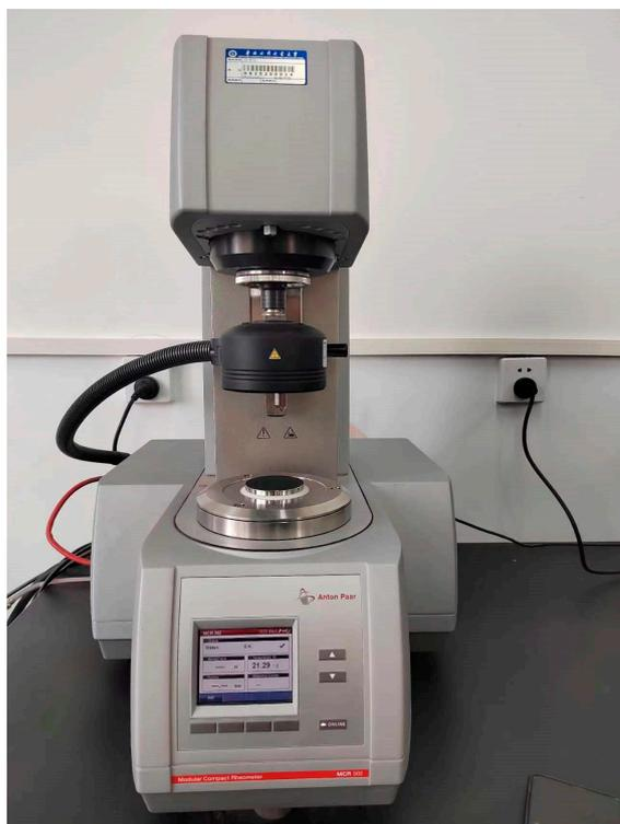
**Figure 26.** The Anton Paar MCR302 rotational rheometer (Anton Paar, Ashland, VA, USA).
