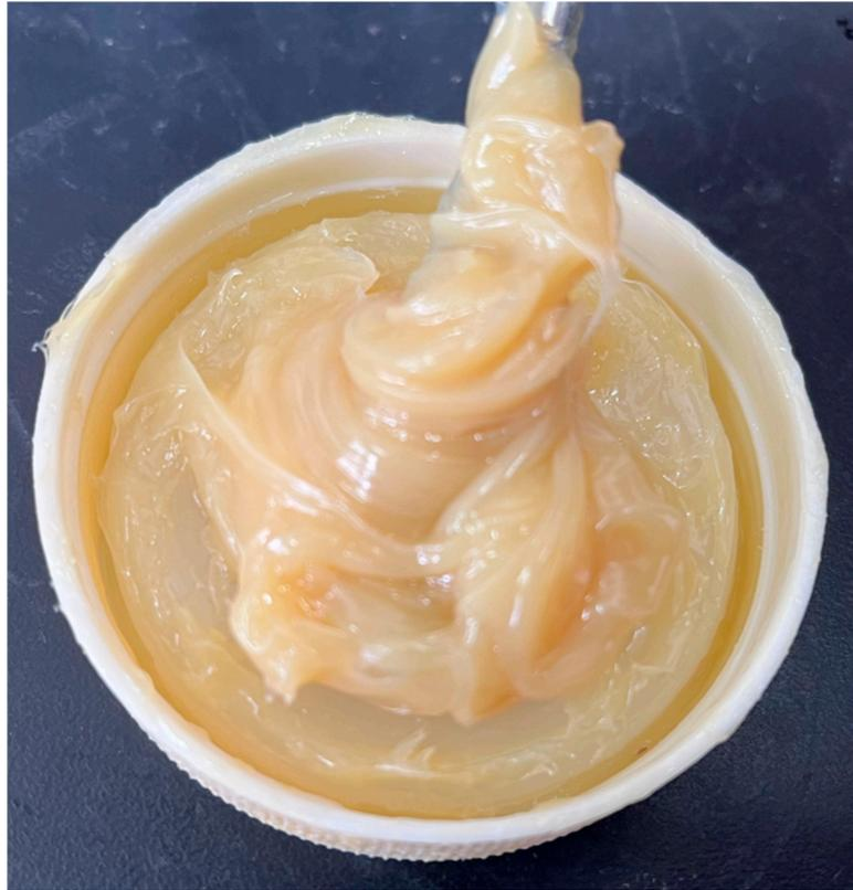
**Figure 28.** The gel state of Mobil SHC 461WT grease.
