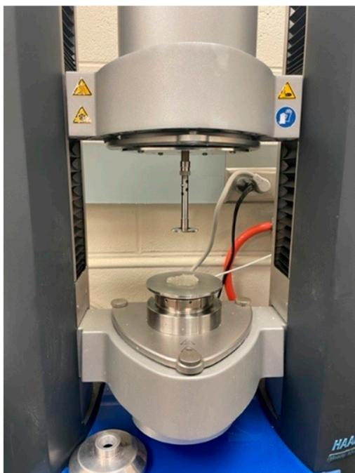
**Figure 20.** Haake MARS III rheometer used to measure the elastic modulus of CMC/PAMBA PPG samples.
