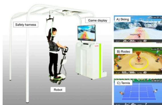
**Figure 1.** Balance Exercise Assist Robot (BEAR). The BEAR moves backward–forward and left–right according to shifts in the operator’s center of gravity. These movements can be incorporated into balance exercises by playing 3 games: (A) a skiing game, which involves using left–right movement; (B) a rodeo game, which requires responses to disturbance stimuli from the BEAR; and (C) a tennis game, which responds to forward–backward movement.
