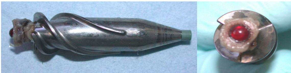
**Figure 1.** HeartMate II impeller: note thrombus formation around the ruby inlet bearing.
