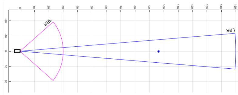
**Figure 3.** Main vehicle millimeter-wave radar detection range. \* Detected objects.
