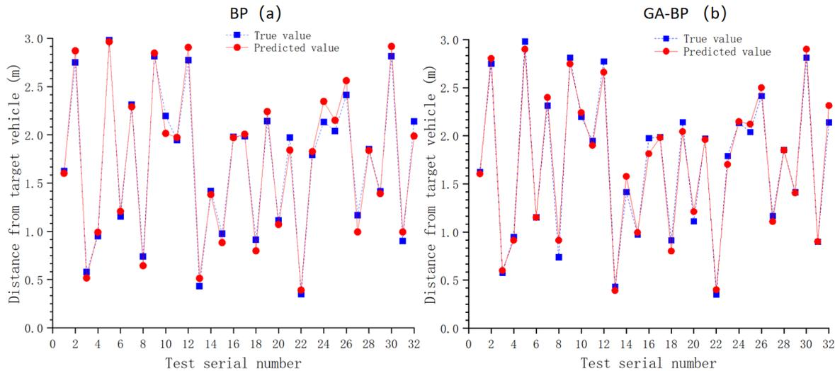
**Figure 13.** BP neural network prediction results (a); modified GA-BP neural network prediction results (b).
