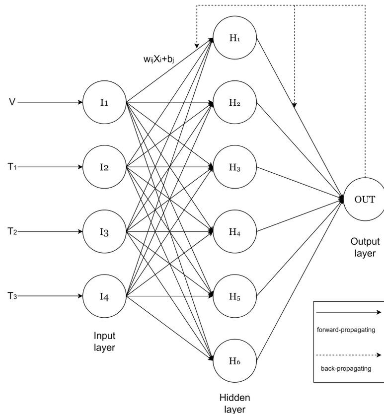
**Figure 4.** The structure diagram of BP neural network after determining the node.
