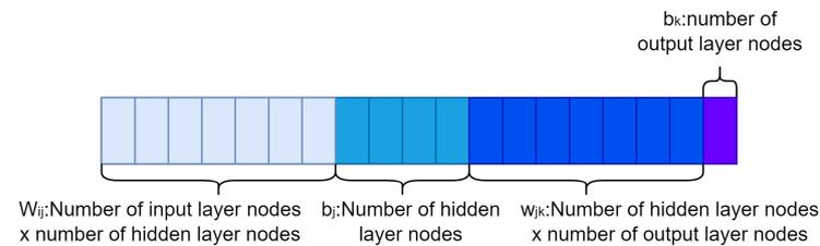
**Figure 6.** Schematic diagram of chromosomes in the genetic algorithm population.
