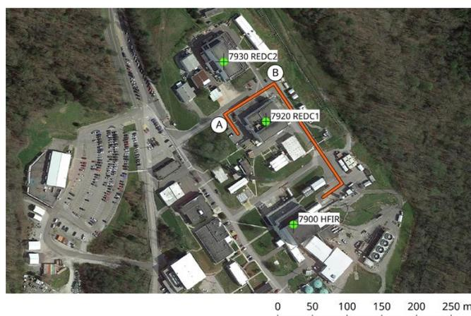
**Figure 1.** Aerial view of MINOS test bed at ORNL with main vehicle transfer route between HFIR and REDC highlighted (orange) and two acoustic sensors indicated (white circles, A and B). Satellite imagery ©2019 Google, used with permission.
