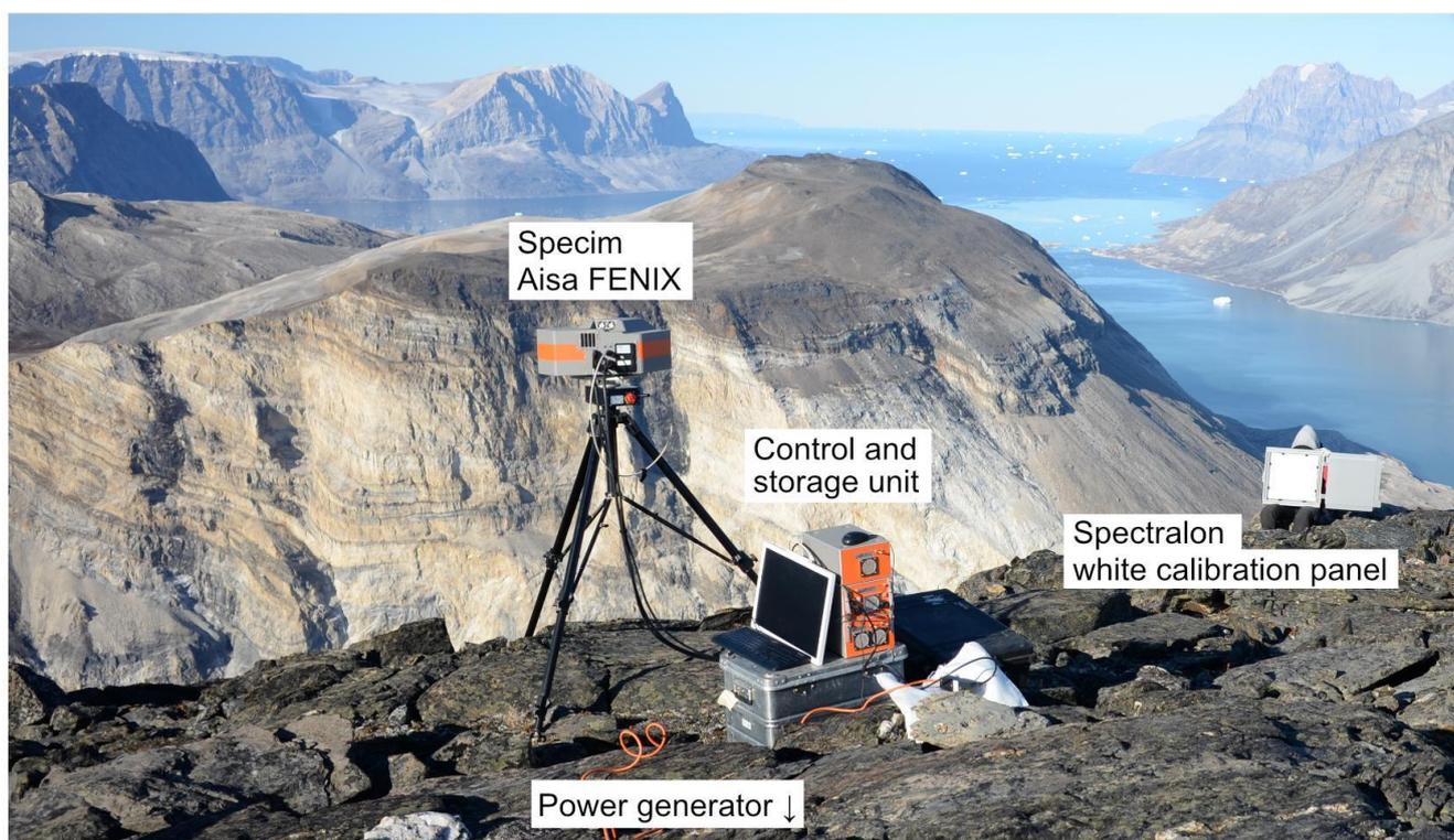
**Figure 3.** Measurement setup for hyperspectral data acquisition.
