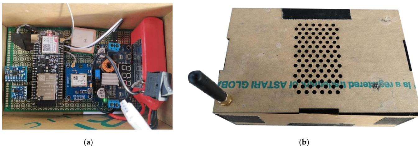
**Figure 6.** Location and orientation logger: (a) electrical component assembly; (b) final packaging with IoT external antenna.
