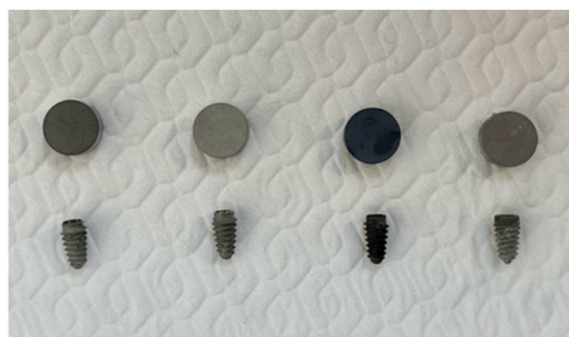
Figure 1. Manufactured disks and implants of the experimental surface groups.
