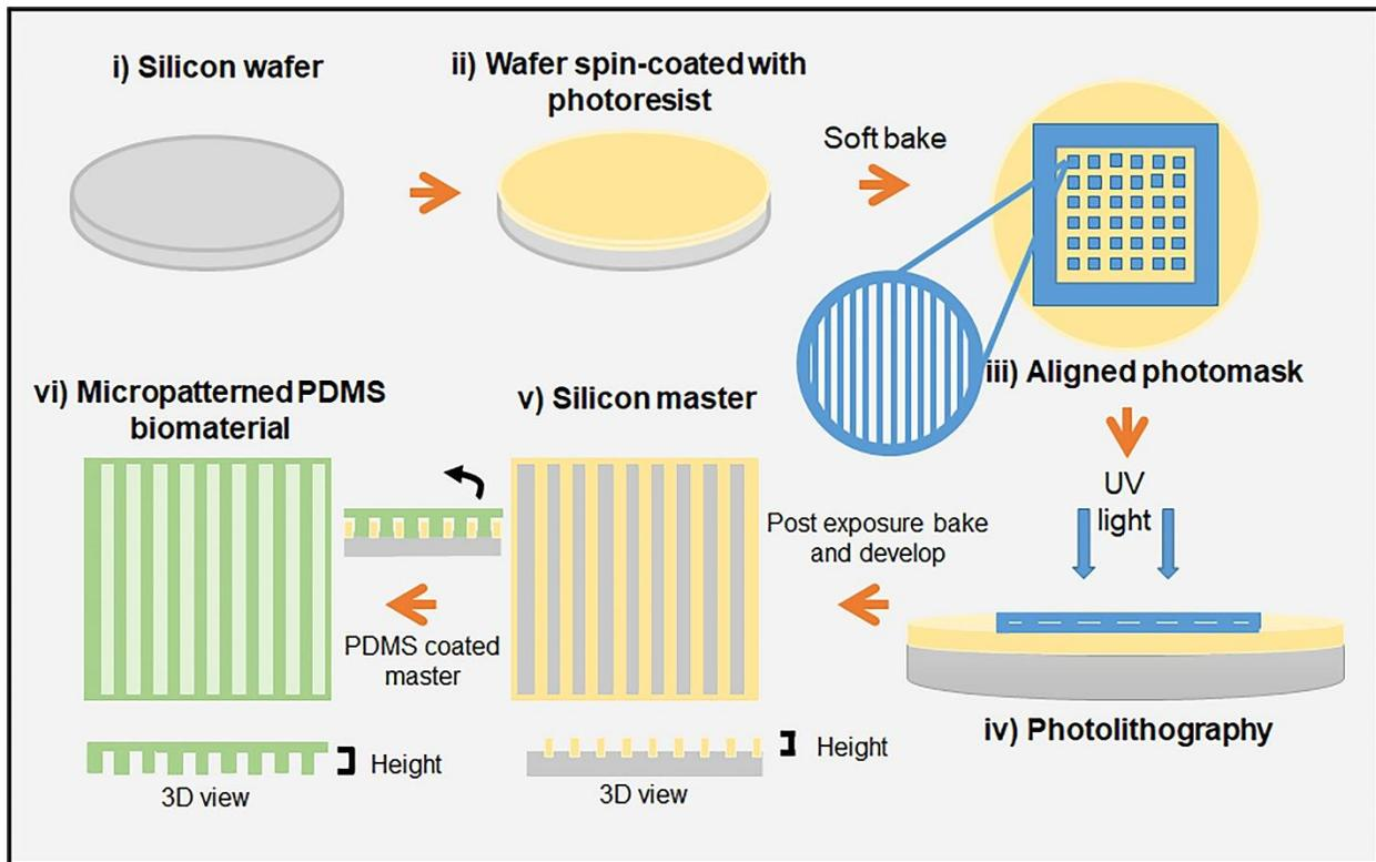
**Figure S1.** Soft lithography protocol for fabrication of micropatterned PDMS biomaterial. The photoresist viscosity and parameters for spin-coating speed, soft bake temperature, photolithography exposure, and post exposure temperature were dependent on the desired three-dimensional pattern height.
