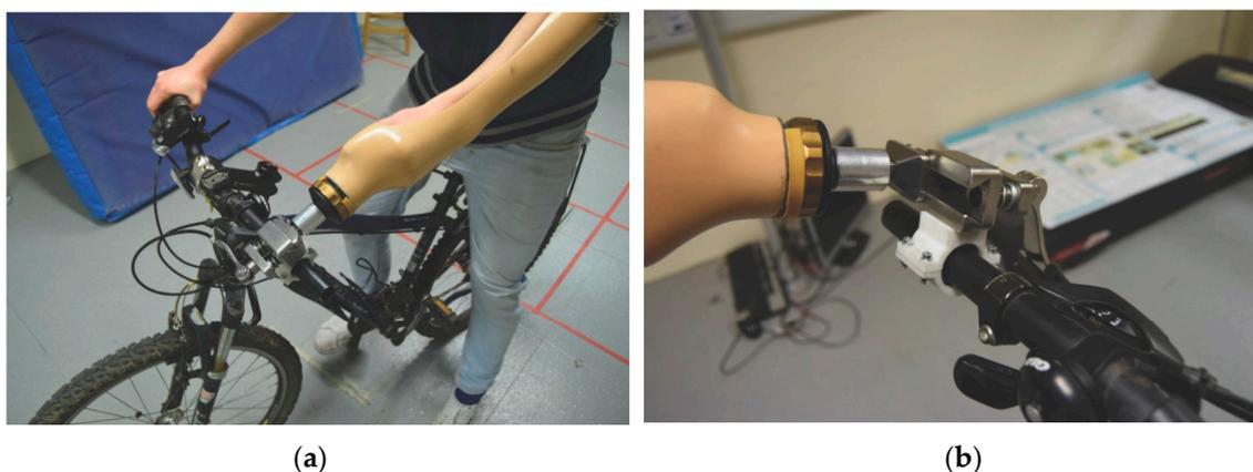
**Figure 9.** Practical experimentation: (a) Volunteer on bicycle; (b) Prosthetic hand release test.
