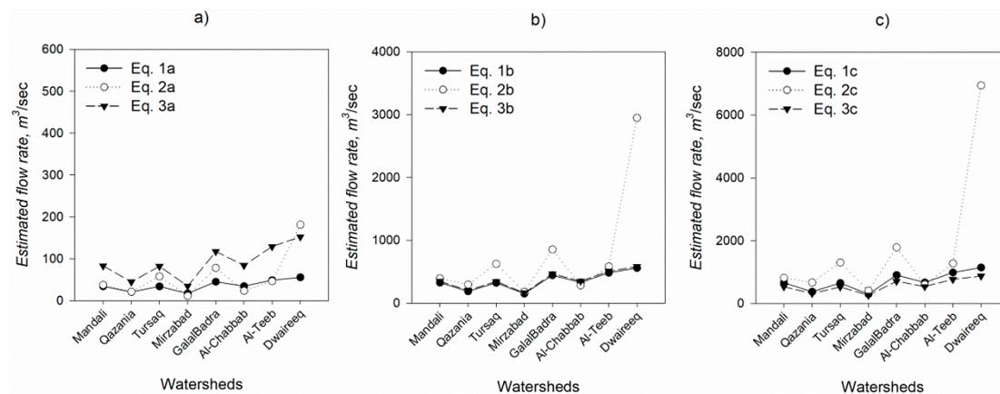
**Figure 5.** Comparison of estimated runoffs using empirical equations of Arizona regions adopted by United States Geological Survey (USGS) for the eight watersheds of: (a) 2-year return period, (b) 25-year return period, and (c) 100-year return period.
