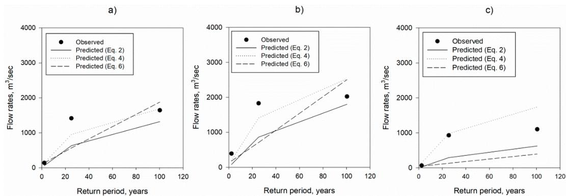
**Figure 8.** Comparison between observed and predicted flow rates at the 2-, 25-, and 100-year return periods for the three streams: (a) Tursaq, (b) Galal Badra, and (c) al-Chabbab.
