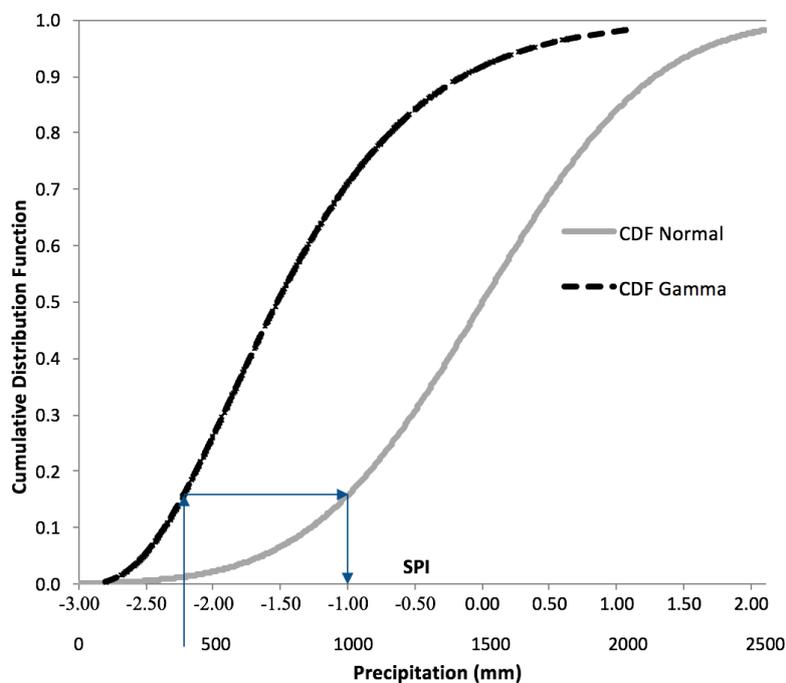
Figure 3. Transformation cumulative distribution function (CDF) gamma to CDF. Adapted from [1].
