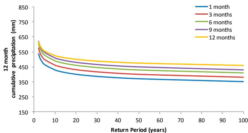
**Figure 7.** Regionalized Severity-Duration-Frequency (SDF) curves for semi-arid climate influence in Minas Gerais.
