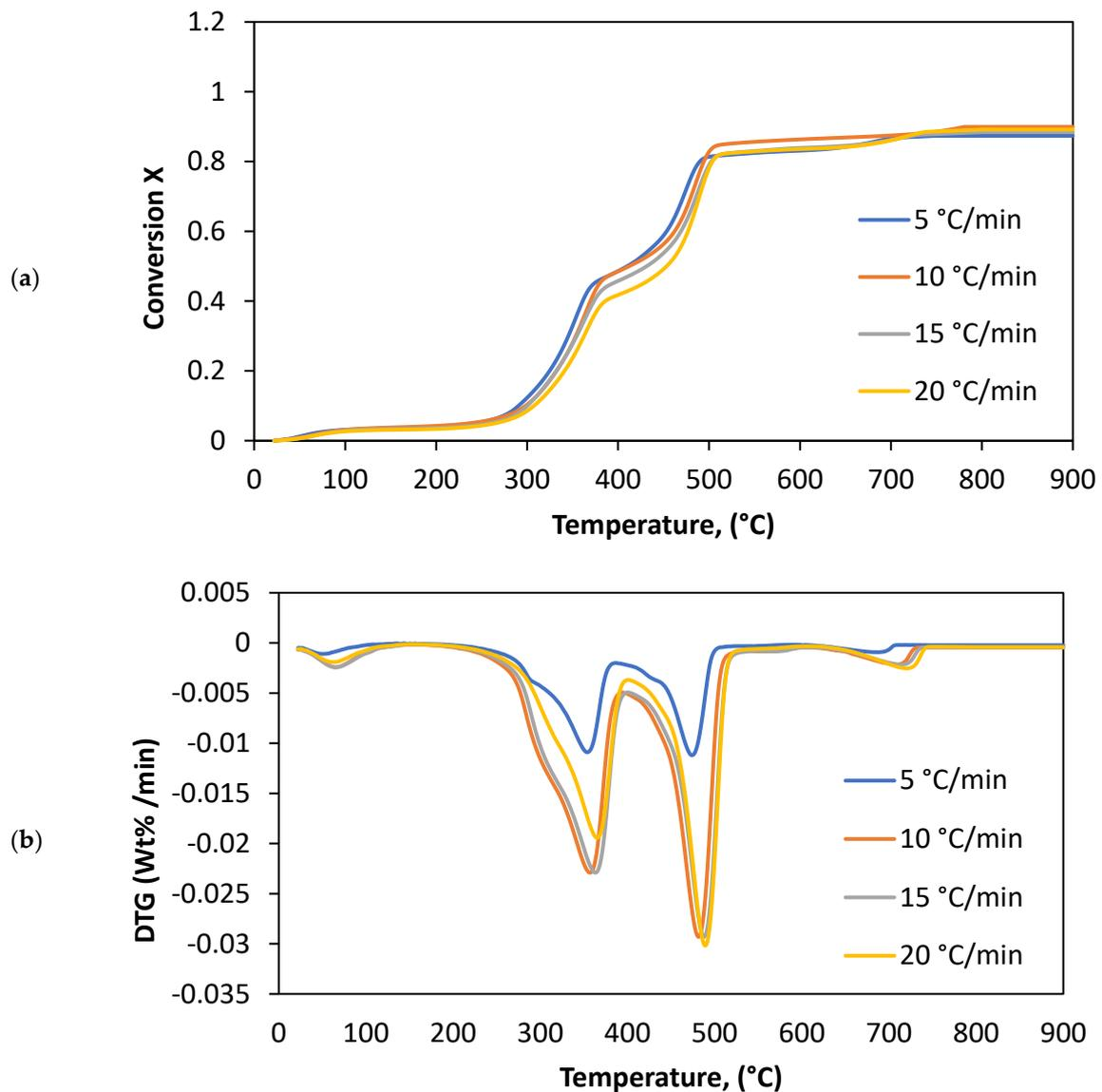
Figure 2. The effect of the heating rate in CO<sub>2</sub>: (a) conversion degree and (b) DTG weight loss.
