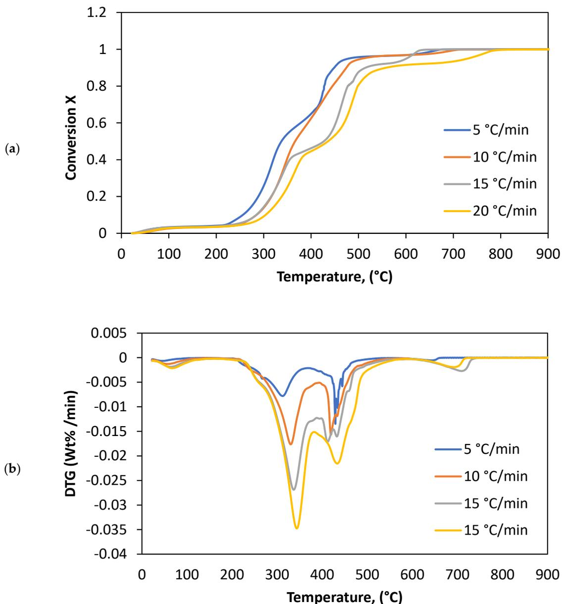
**Figure 3.** The effect of the heating rate in air: (a) conversion degree and (b) DTG weight loss.
