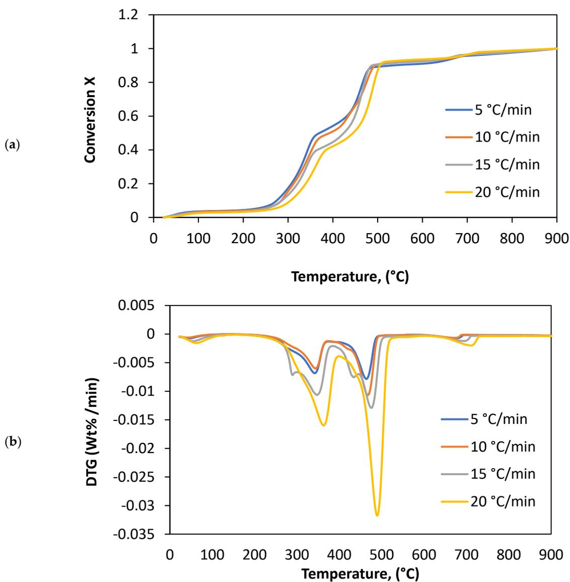
Figure 1. The effect of the heating rate in N<sub>2</sub>: (a) conversion degree and (b) DTG weight loss.
